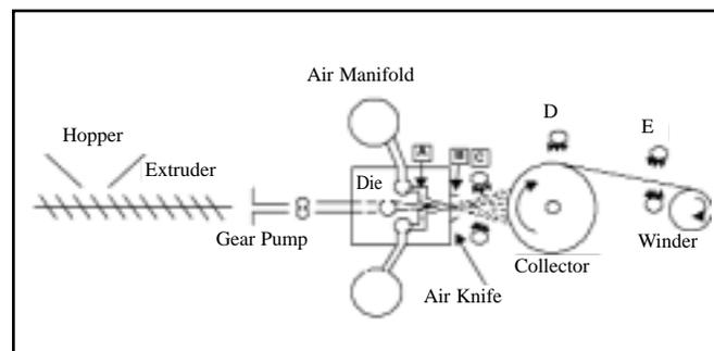
and bottom air knives, respectively. The spacing between two pins was 1.27 cm. Two solid bars, each having a diameter of 2.54 cm, were located 3.7 cm away from the center line of the air gap and also 3.7 cm from the air knife measured from the center of the bar. The bar was subjected to positive or negative high voltage while the pins were grounded with the die body. The fibers were charged at the die exit when they were still in molten stage by electric field force or by aerodynamic force.
