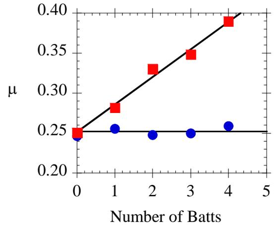
FIGURE 5. The friction coefficient for the polyester knit fabric resting on 0-4 polyester batts. Symbols and lines are the same as in Figure 4.
