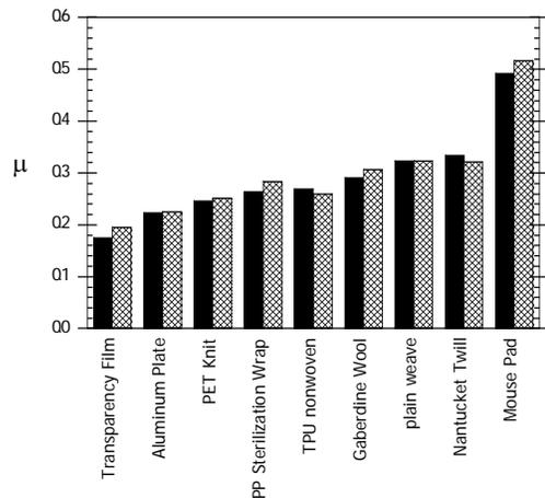
FIGURE 3. Friction coefficient measured by the guarded, G, sled (solid) and the conventional sled, S, (crosshatched) for several non-deformable substrates.
