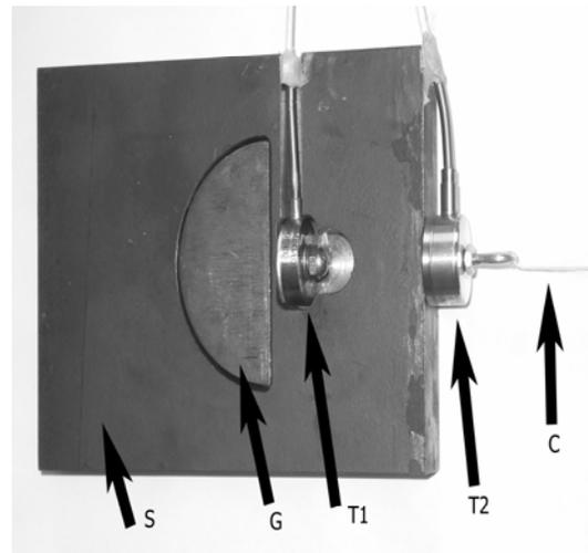
FIGURE 1. The compound sled that forms the guarded friction meter is shown. The conventional sled, S, is pulled by cord, C, and tension load transducer,  $T_2$ , which measures the force,  $F_c$ , required to pull the compound sled. S, in turn, pulls the guarded sled, G, via compression load transducer,  $T_1$ , which measures the force,  $F_g$ , required to pull only the guarded sled. The guarded sled floats freely within the conventional sled, restrained only by  $T_1$ .
