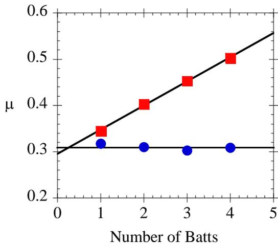
FIGURE 4. Friction coefficients of 1-4 polyester batts. The same batt is always in contact with the sled. Circles are friction coefficients obtained from the guarded sled while the squares are from the conventional sled. The horizontal line represents the
