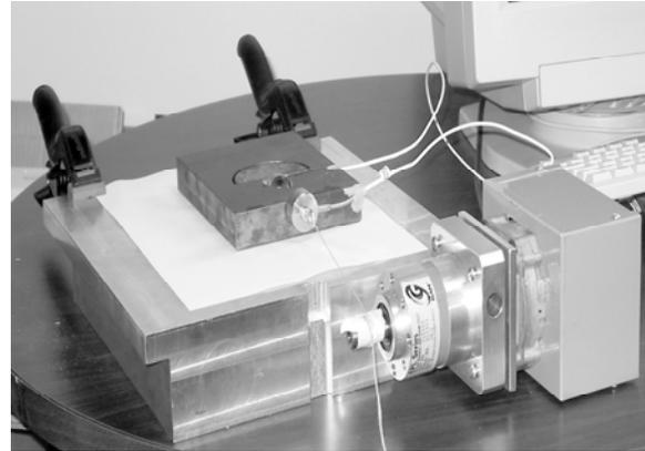
FIGURE 2. Fabric under test (white object) is placed on aluminum support block and its back edge clamped to the aluminum plate. The guarded friction device is placed on the test specimen, the towing cord is attached to the motor drive and the drive started.
