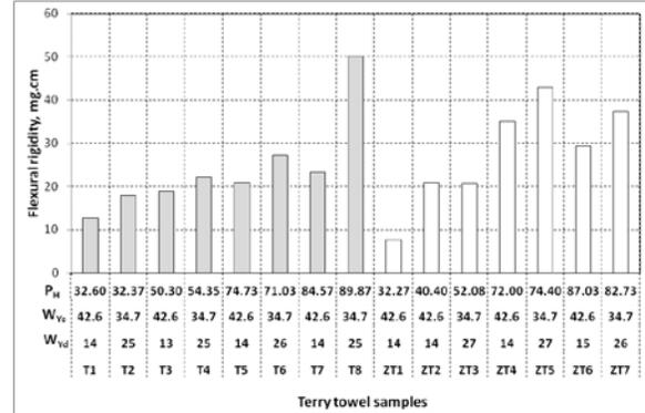
FIGURE 2. Flexural rigidity test results; P<sub>H</sub>= pile height (mm), W<sub>Yc</sub> = weft yarn count (tex), W<sub>Yd</sub>= weft density (weft/cm), T= towels with twisted pile yarn, ZT=towels with twistless pile yarn.
