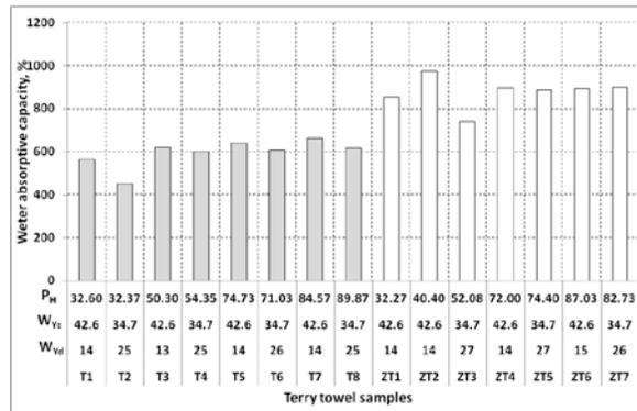
FIGURE 4. Water absorptive capacity of terry towel fabrics;  $P_H$ = pile height (mm),  $W_{Yc}$  = weft yarn count (tex),  $W_{Yd}$ = weft density (weft/cm), T= towels with twisted pile yarn, ZT=towels with twistless pile yarn.
