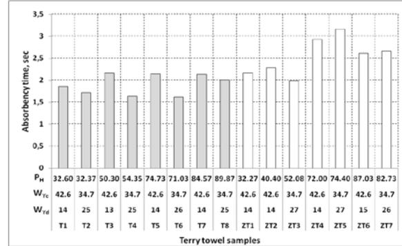
FIGURE 3. Water absorbency time;  $P_H$ = pile height (mm),  $W_{Yc}$  = weft yarn count (tex),  $W_{Yd}$ = weft density (weft/cm), T= towels with twisted pile yarn, ZT=towels with twistless pile yarn.
