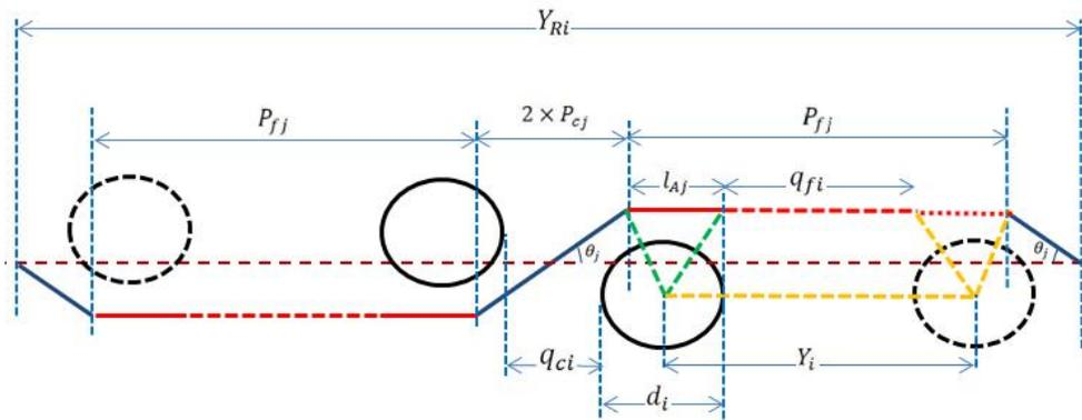
FIGURE 4. Geometrical parameters in weave repeat.
