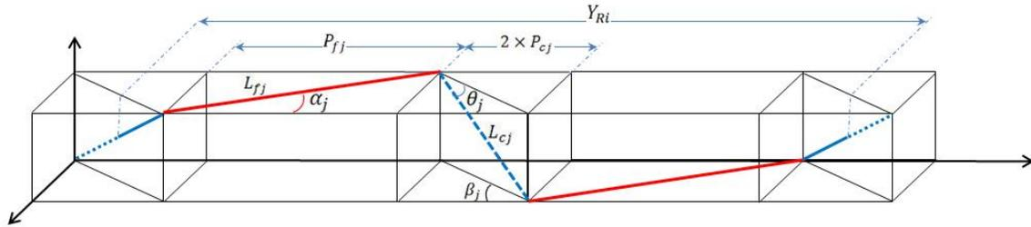
FIGURE 5. Three Dimensional Weave Repeat Geometry.
