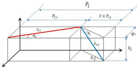
FIGURE 6. Three Dimensional Unit Cell Geometry.
