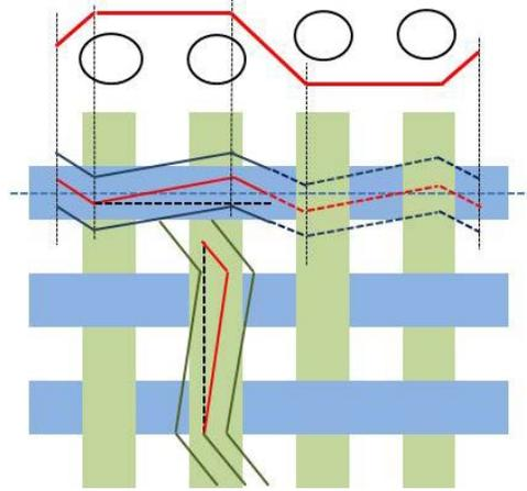
FIGURE 3. Skewed straight line yarn path.
