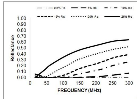
FIGURE 5. Reflectance of nonwoven fabrics with different percentage of stainless steel fibers between 15-300MHz.
