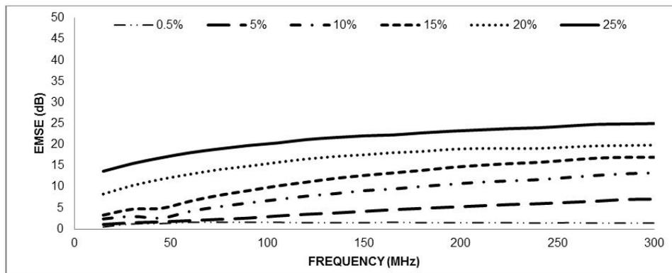
FIGURE 11. Electromagnetic Shielding (EMSE) of Nonwoven Fabrics with Different Percentage of Stainless Steel Fibers between 15-300MHz.
