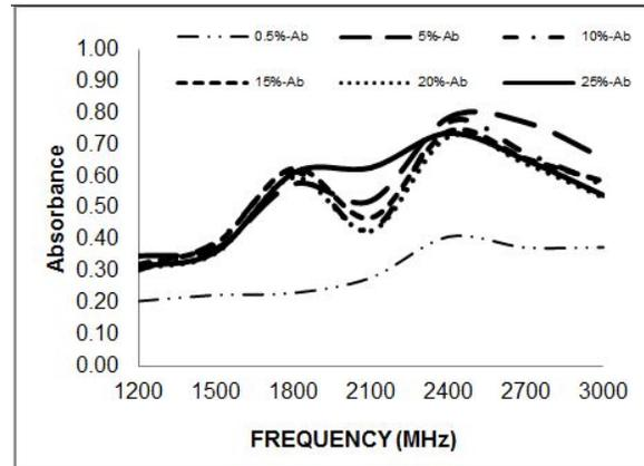
FIGURE 10. Absorbance of Nonwoven Fabrics with Different Percentage of Stainless Steel Fibers Between 1200-3000Mhz.
