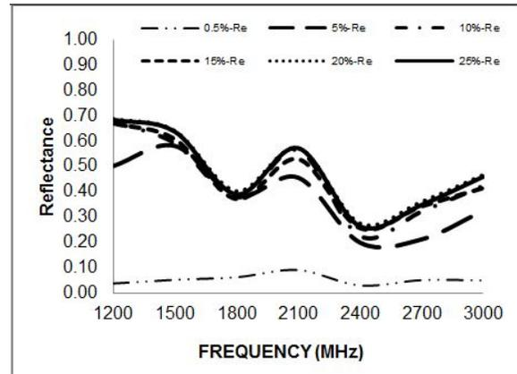
FIGURE 9. Reflectance of Nonwoven Fabrics with Different Percentage of Stainless Steel Fibers Between 1200-3000MHz.
