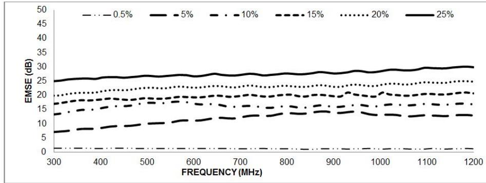
FIGURE 12. Electromagnetic Shielding (EMSE) of Nonwoven fabrics with Different Percentage of Stainless Steel Fibers Between 300-1200MHz.
