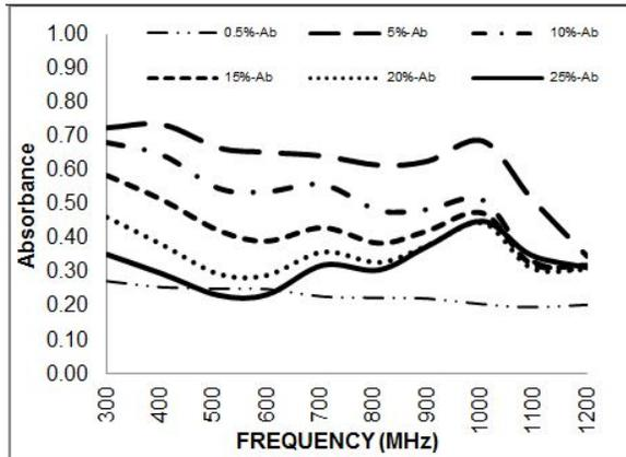
FIGURE 8. Absorbance of Nonwoven Fabrics with Different Percentage of Stainless Steel Fibers between 300-1200MHz.
