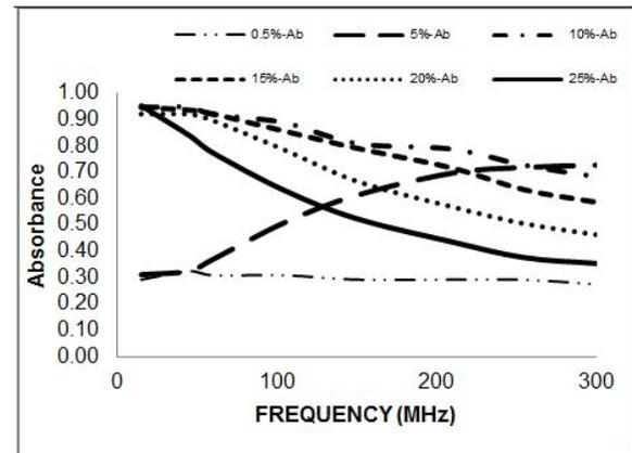
FIGURE 6. Absorbance of nonwoven fabrics with different percentage of stainless steel fibers between 15-300mhz.
