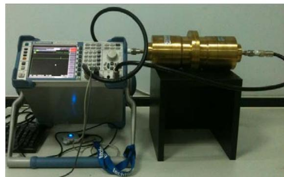
FIGURE 2. Set up of EMSE Testing Apparatus.
