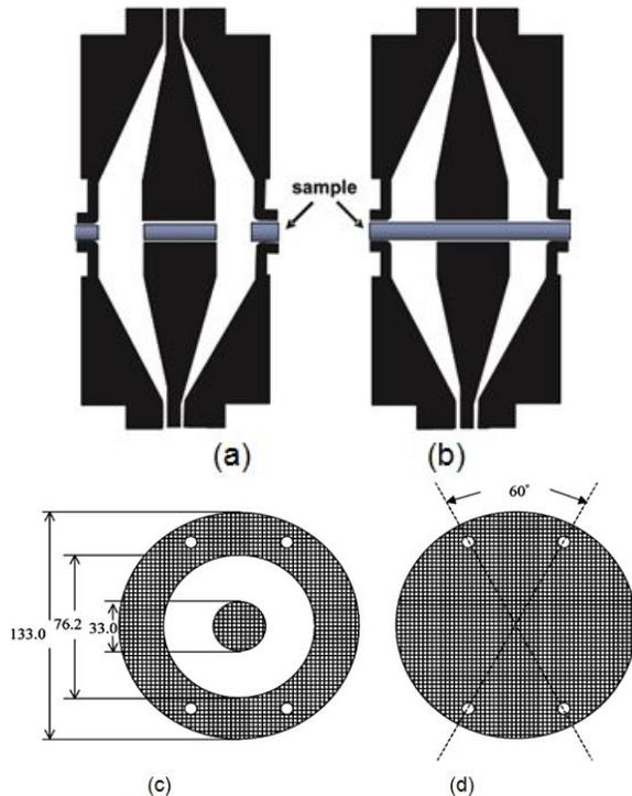
FIGURE 3. A cross-section of the shielding effectiveness test fixture (a) reference sample in the jig and (b) load sample in the jig. Specific dimensions of the specimens for shielding effectiveness measurement (unit: mm), (c) Reference sample (d) Load sample.
