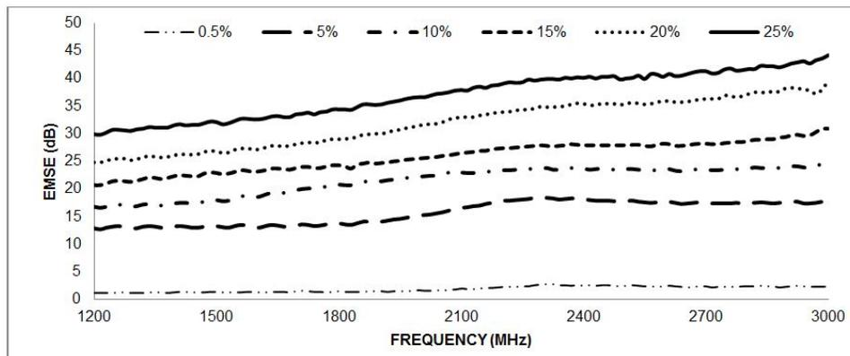
FIGURE13. Electromagnetic Shielding (EMSE) of Nonwoven Fabrics with Different Percentage of Stainless Steel Fibers between 1200-3000MHz.
