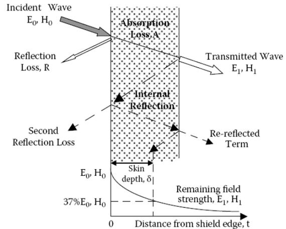
FIGURE 1. Graphical Representation of EMI Shielding.
