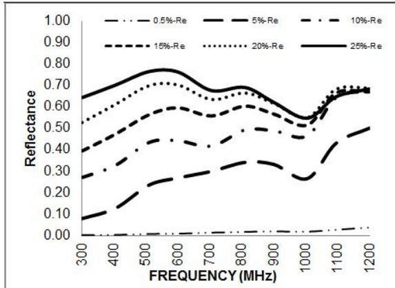
FIGURE 7. Reflectance of Nonwoven Fabrics with Different Percentage of Stainless Steel Fibers Between 300-1200MHz.
