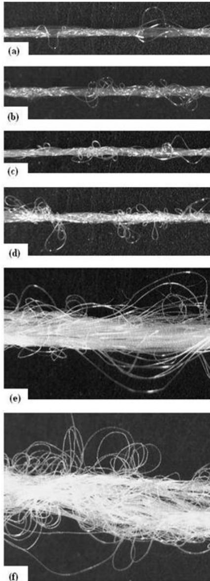
FIGURE 2. Optical microscopy images of the yarns: (a)PET15, (b)PET30, (c)PBT15, (d)PBT30, (e)Vectran15, (f)Vectran30.
