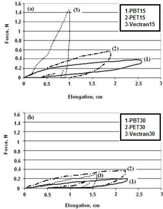
FIGURE 4. Recovery cycles: (a)PET15, PBT15, Vectran15, (b)PET30, PBT30, Vectran30.
