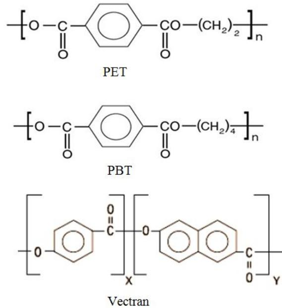
FIGURE 3. Molecular structures of the samples.
