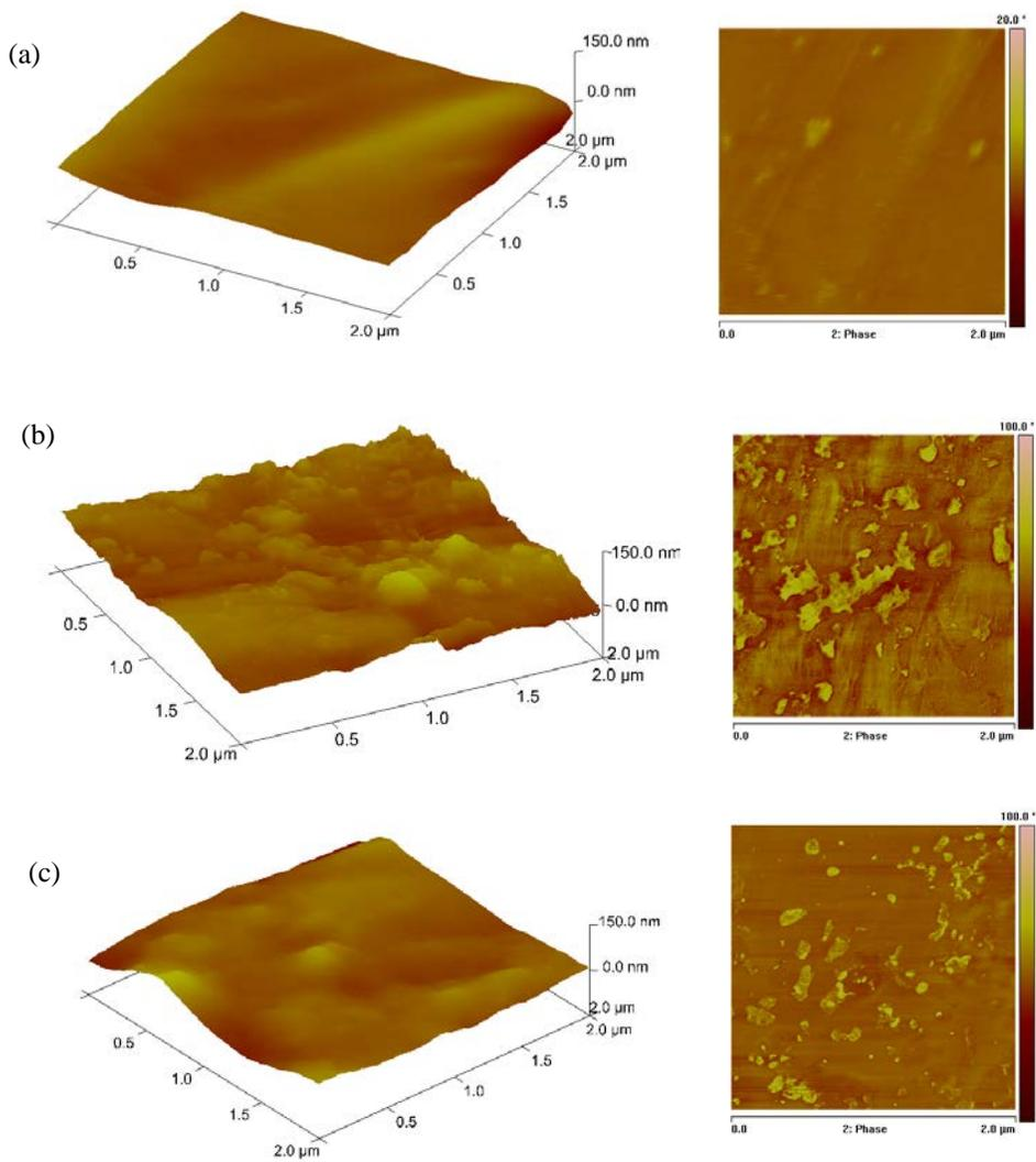
FIGURE 3. AFM images of the samples: a) PET, b)Antistatic PET, c) Antibacterial PET.
