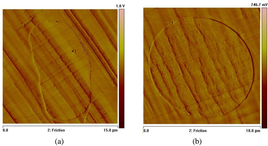
FIGURE 4. AFM images of the cross sections of the fibers: a)Antibacterial PET friction, b)Antistatic PET friction.
