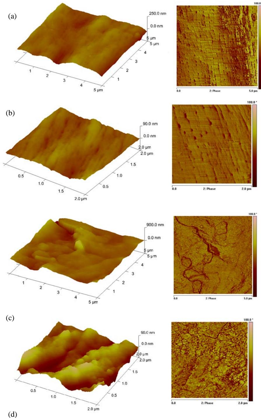
FIGURE 2. AFM images of the samples: a) Cotton topography and phase (5 μm × 5 μm), b) Cotton topography and phase (2 μm × 2 μm), c) Wool topography and phase (5 μm × 5 μm) d) Wool topography and phase (2 μm × 2 μm).
