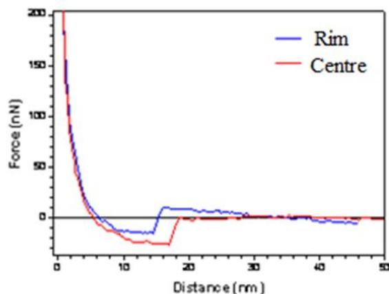
FIGURE 5. Force-distance curve of trilobal PET ( Taken from 2 different places on the fiber cross-section. Near the surface and near the centre).
