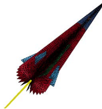
FIGURE 4. (color online) surface mesh of the rescue parachute canopy.
