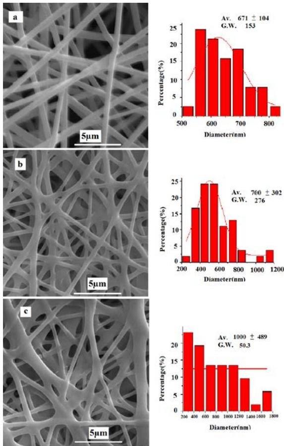
FIGURE 6. Morphology of as-spun PVA/ NiO-GDC mats for the samples obtained with a 10% (w) polymer solution at a traveling distance of 100 mm, needle diameter of 0.6 mm, voltage of 10 kV and flow rate of (a): 0.1 ml h<sup>-1</sup>, (b):0.3 ml h<sup>-1</sup>, (c): 0.5 ml h.
