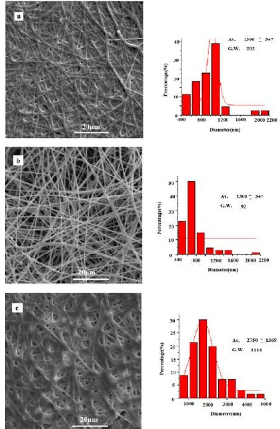
FIGURE 5. Morphology of the as-spun PVA/ NiO-GDC mats for the samples obtained for a 10% (w) polymer solution, and a needle diameter of 0.5 mm, flow rate of 0.1 ml h<sup>-1</sup>, a voltage of 15 kV and a distance between the needle tips to collector of (a) 80 mm, (b) 100 mm, (c) 150 mm.
