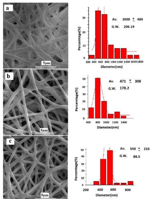
FIGURE 4. Morphology of the as-spun PVA/NiO-GDC mats for the samples obtained with a 10% (w) polymer solution at a traveling distance of 100 mm, needle diameter of 0.6 mm, flow rate of 0.1 ml h<sup>-1</sup> and a voltage of (a) 8 kV, (b) 10 kV, (c) 15 kV.
