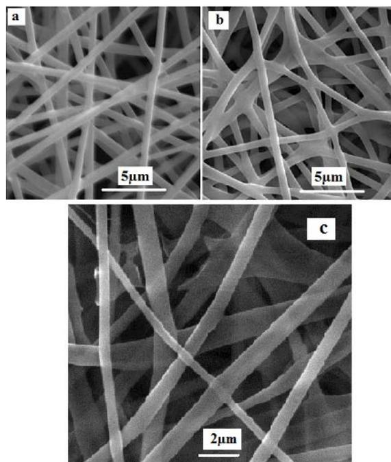
FIGURE 1. Morphology of the as-spun PVA/NiO-GDC fibers obtained with traveling distance of 100 mm, needle diameter of 0.6 mm, voltage of 10kV and flow rate of 0.1 ml h<sup>-1</sup> and a polymer concentration with: (a) 8 %w, (b) 10 %w, (c) 15 %w. (SEM MAG: 10 kx).
