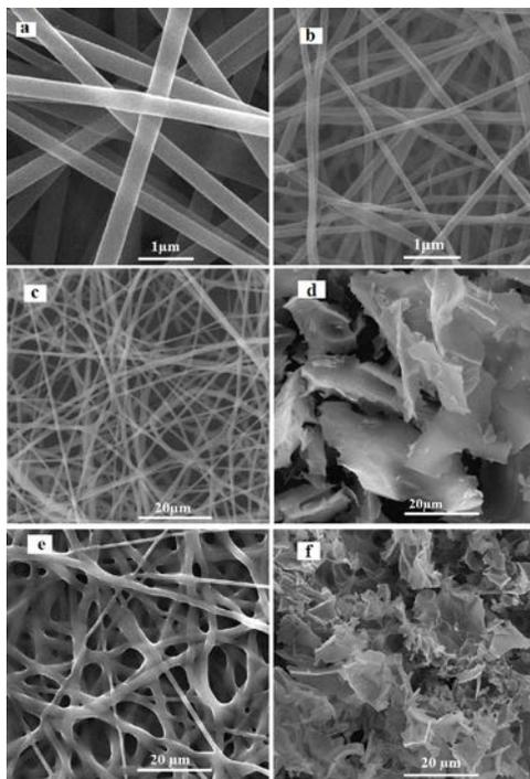
FIGURE 2. Morphology of the samples obtained with a 10% (w) polymer solution at a traveling distance of 100 mm, needle diameter of 0.6 mm, voltage of 10 kV, flow rate of 0.1 ml h<sup>-1</sup>, and cationic concentration (a,b): 0.5 M, (c,d): 1 M, (e,f): 2 M before and after calcinations in right and left, respectively.
