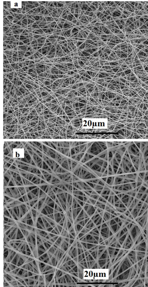
FIGURE 7. Morphology of the as-spun PVA/ NiO-GDC mats for the samples obtained with a 10% (w) polymer solution at a traveling distance of 100 mm, voltage of 10 kV, flow rate of 0.1 ml h<sup>-1</sup> and the diameter of the needle (a) 0.6 mm, (b) 0.8 mm.(SEM MAG:2kx).
