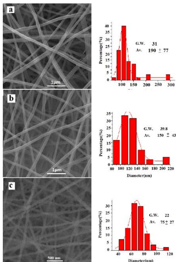
FIGURE 3. Morphology of the NiO-GDC nanofibers calcined at (a):800 °C, (b): 900 °C, (c): 1000 °C.
