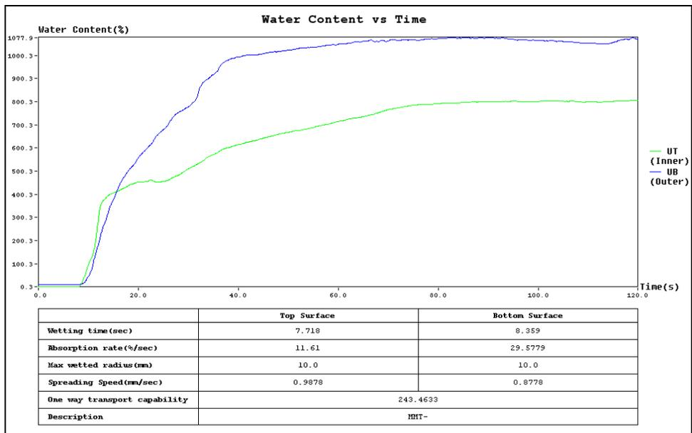
FIGURE 7. MMT results for the fabrics produced by channeled PES yarns after moisture management finishing.
