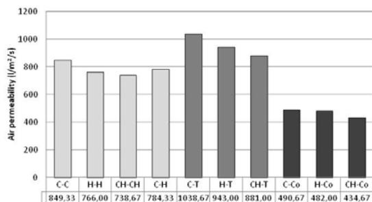
FIGURE 2. Air permeability test results.
