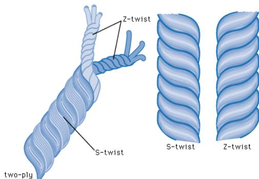
FIGURE 1. Plying of yarns [4].
