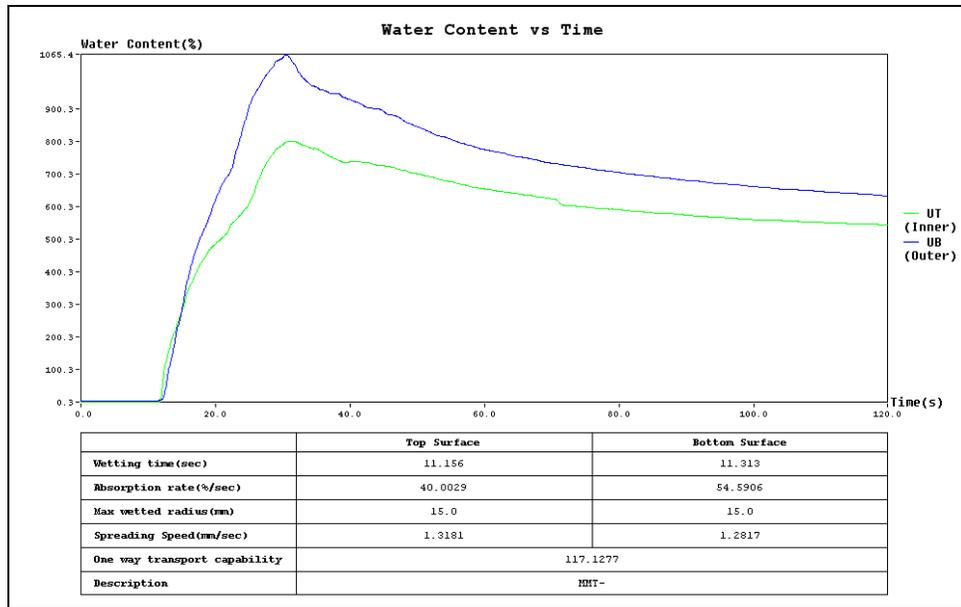
FIGURE 8. MMT results for the fabrics produced by hollow PES yarns after moisture management finishing.
