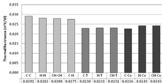
FIGURE 3. Thermal resistance test results.
