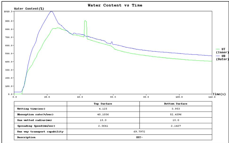
FIGURE 9. MMT results for the fabrics produced by channeled PES-lyocell yarns after moisture management finishing.
