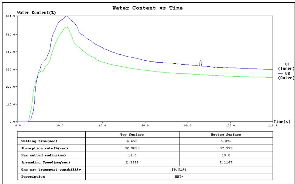
FIGURE 10. MMT results for the fabrics produced by channeled PES-cotton yarns after moisture management finishing.
