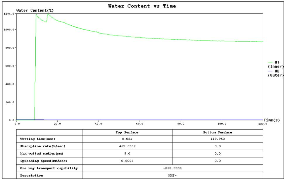
FIGURE 6. MMT results for the fabrics produced by channeled PES yarns before moisture management finishing.
