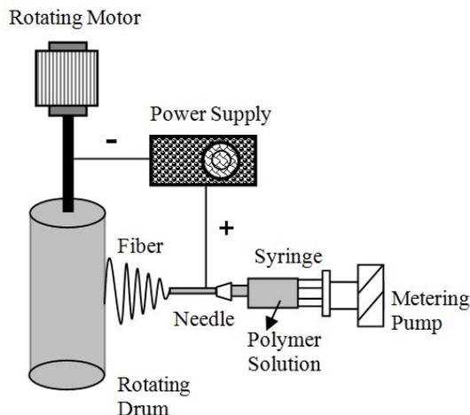
FIGURE 1. System set-up of the electro-spinning unit for manufacturing PSA fibers.
