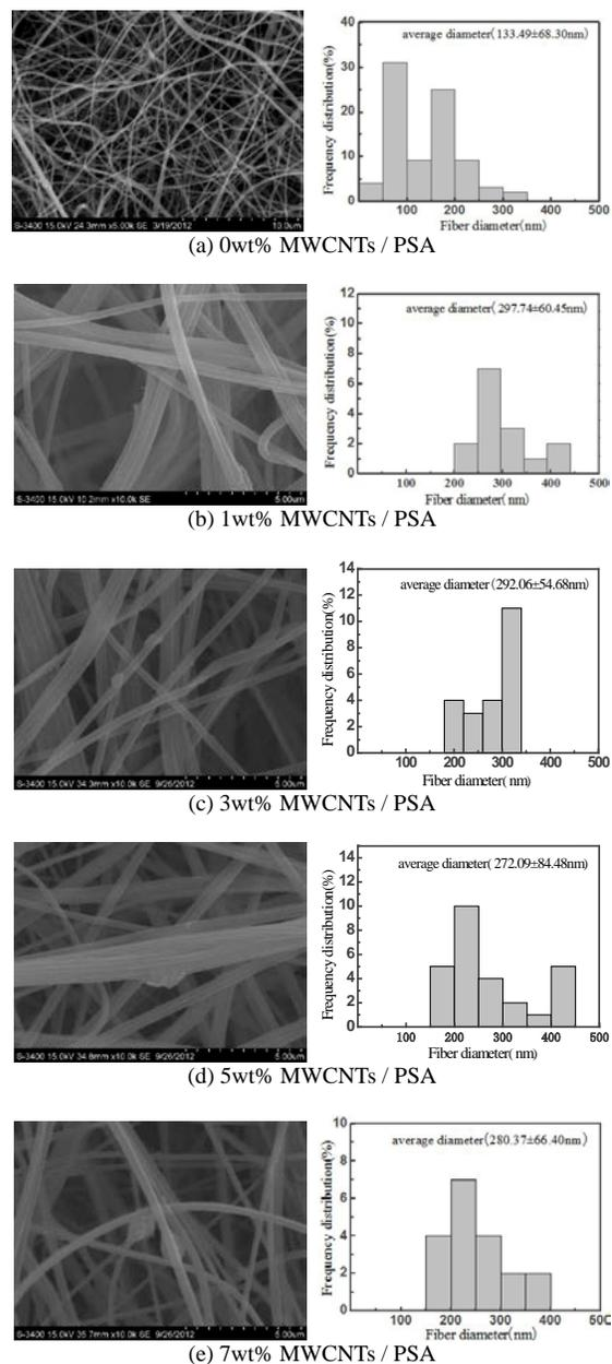
FIGURE 2. SEM images and diameter distribution of 12% PSA electrospun fibers with different MWCNT concentrations.
