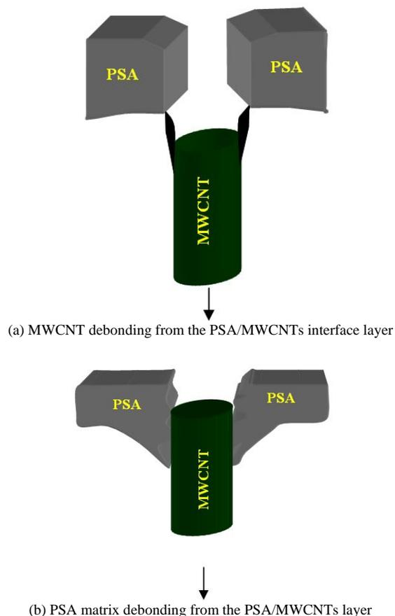
FIGURE 8. The Failure Model of the PSA/MWCNTs composite fibers.
