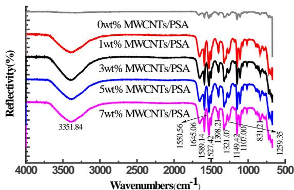
FIGURE 5. FTIR Curves of the electrospun PSA/MWCNTs fibers.
