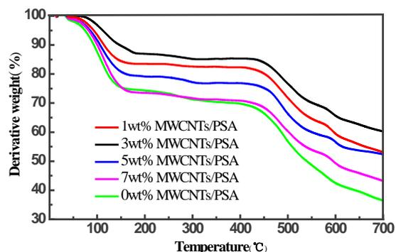
FIGURE 9. The TG curves of PSA/MWCNTs fibers with different MWCNT concentrations.
