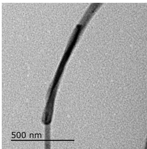
FIGURE 3. TEM images of MWCNTs/PSA electrospun fibers with 3% MWCNTs.
