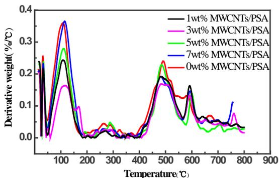
FIGURE 10. The DTG curve of PSA/MWCNTs fibers with different MWCNT concentrations.
