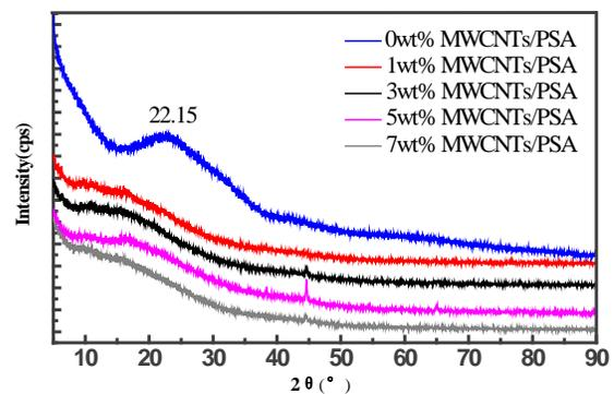
FIGURE 4. The X-ray Diffraction Intensity Curve of the PSA/MWCNTs Fibers.
