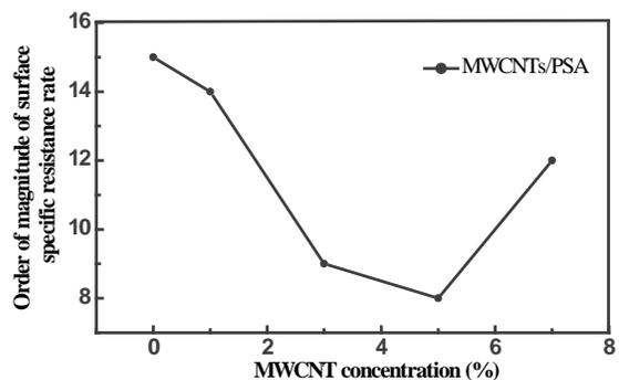
FIGURE 6. The surface specific resistance rate of PSA/MWCNTs fibers prepared with different MWCNT concentrations.
