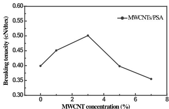
FIGURE 7. The breaking tenacity of the electrospun PSA/MWCNTs fibers with different MWCNT concentrations.
