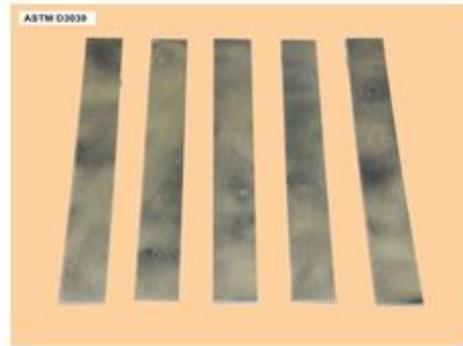
(a)CFRP Plain Coupon
