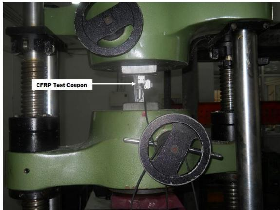
FIGURE 6. UTM Test Setup.
