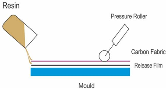
FIGURE 3. Schematic Diagram showing the Hand lay-up process.
