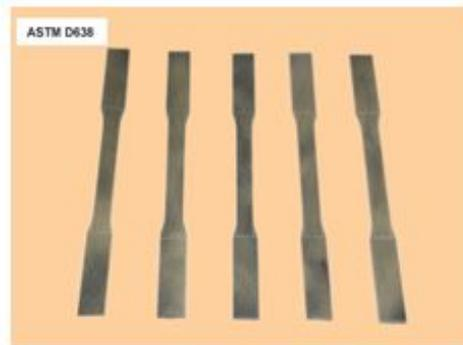
(b)CFRP Dumb Bell Coupon
