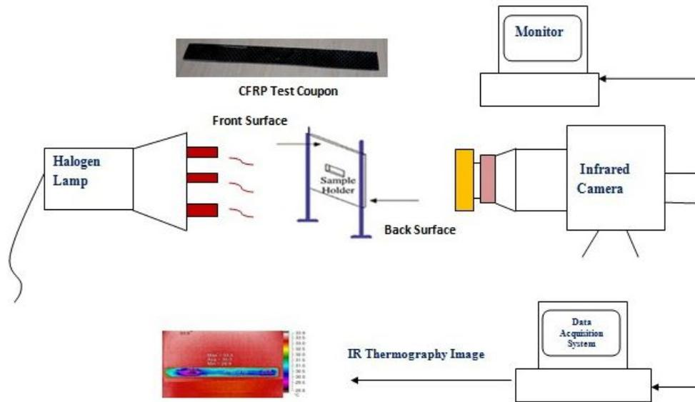
FIGURE 5. Schematic Representation of IR Thermography testing technique for Composites
