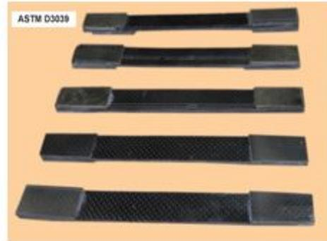
(c)CFRP Coupon with End Tab
