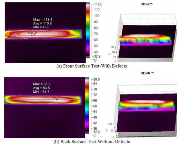
FIGURE 9. IR Thermography of Image of Test No. CFRP2.
