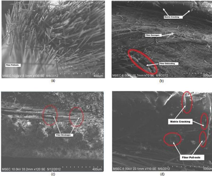
FIGURE 14. SEM Photographs of carbon fabric/epoxy composite.
