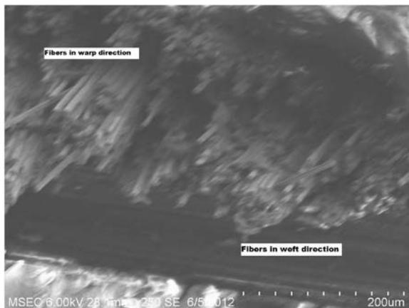
FIGURE 4. SEM image showing the carbon fabric/epoxy composite.
