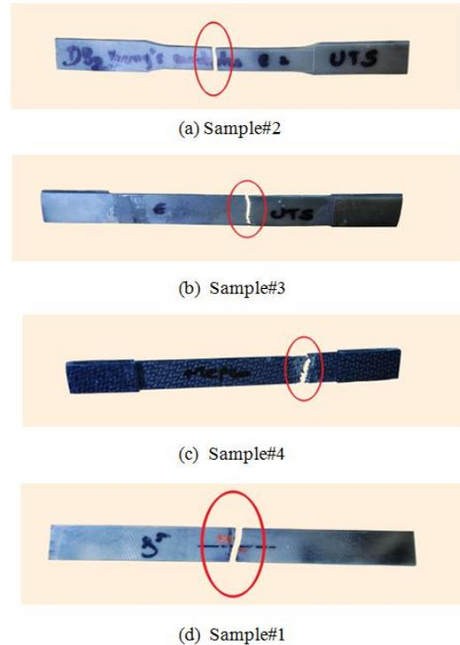
FIGURE 10. Failure mode of Carbon Fabric/Epoxy Composite.
