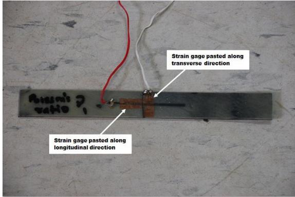
FIGURE 7. Poisson's ratio Testing.
