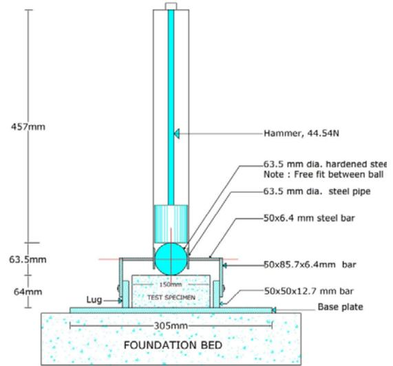
FIGURE 1. Schematic Diagram of the Drop Weight Method Test Setup.
