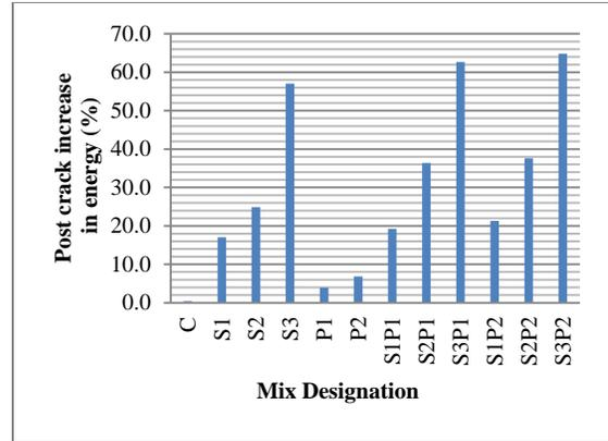
FIGURE 6. Post crack strength Energy for all mixes.
