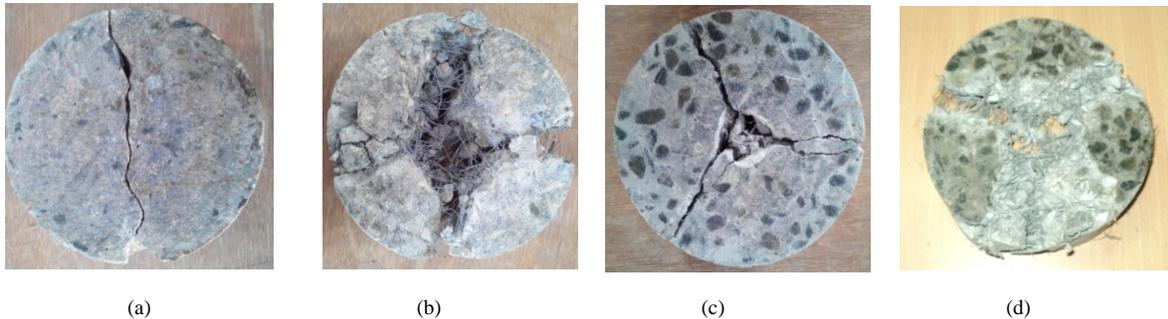
FIGURE 7. Failure pattern of the concrete specimen (a) Control specimen (b) SFRC (c) PFRC (d) SPHFRC.
