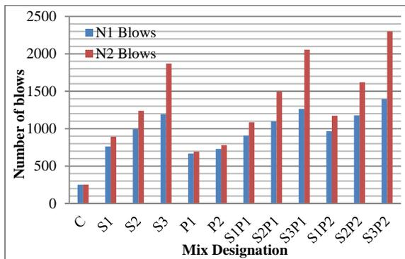
FIGURE 5. Impact resistance at first crack and ultimate failure.
