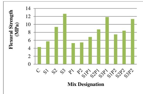
FIGURE 4. Flexural strength at 28 days.
