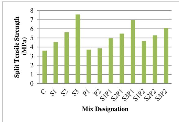
FIGURE 3. Split tensile strength at 28 days.
