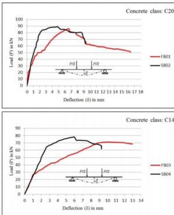
FIGURE 13. Comparison of load-deflection ( $P-\delta$ ) curves for strengthened beams; (a) for C20 class, (b) for C14 class.
