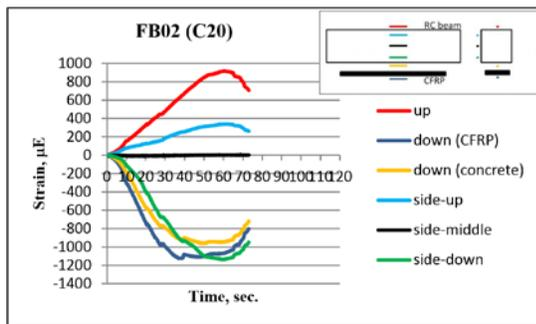
FIGURE 7. The variation of strain with time for beam FB02.
