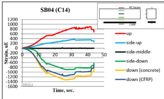
FIGURE 8. The variation of strain with time for beam SB04.
