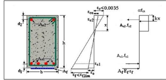
FIGURE 6. Tensile block approach used in the FRP-Analysis Software.
