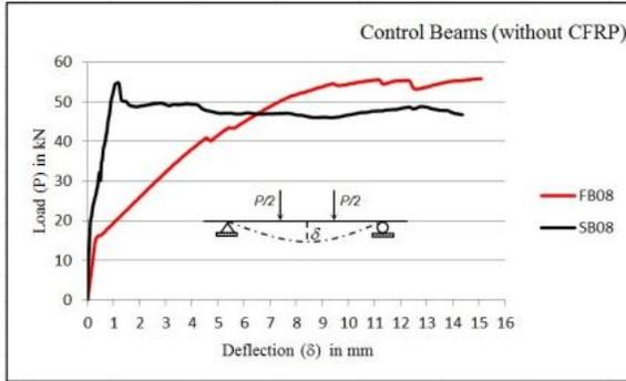
FIGURE 14. Comparison of load-deflection ( $P-\delta$ ) curves for control beams.
