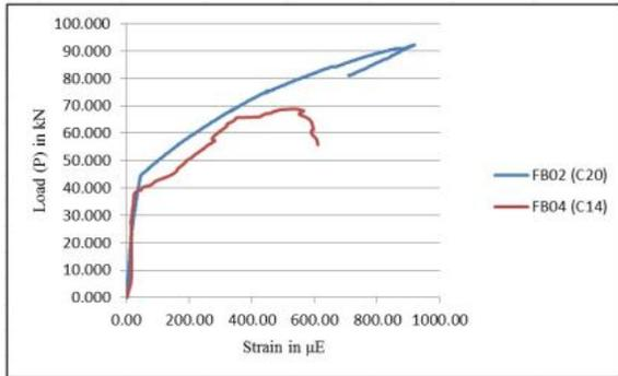
FIGURE 15. Load-deformation relation for beams FB02 and FB04.
