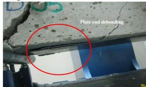
FIGURE 10. Plate end debonding on beam SB05.
