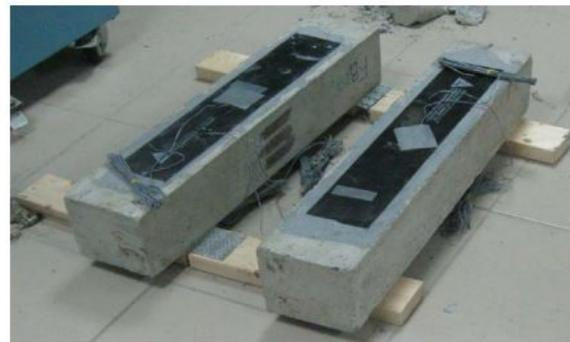
FIGURE 4. The application of CFRP on the lower surface of the beams.
