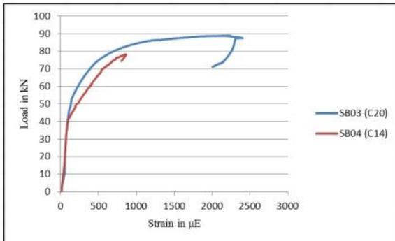
FIGURE 16. Load-deformation relation for beams SB03 and SB04.
