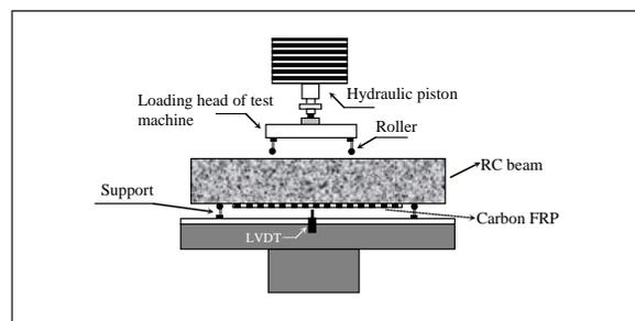
FIGURE 2. The experimental set-up and its instrumentation.
