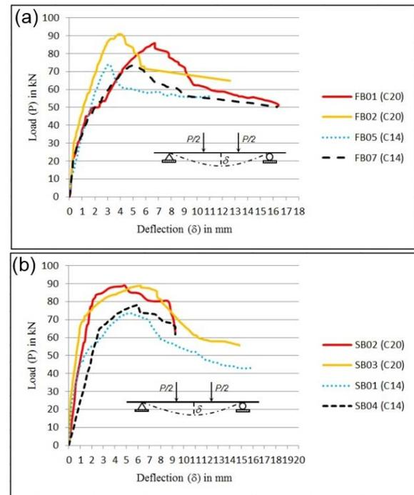
FIGURE 12. Comparison of load-deflection ( $P-\delta$ ) curves for strengthened beams; (a) FB Series, (b) SB Series.
