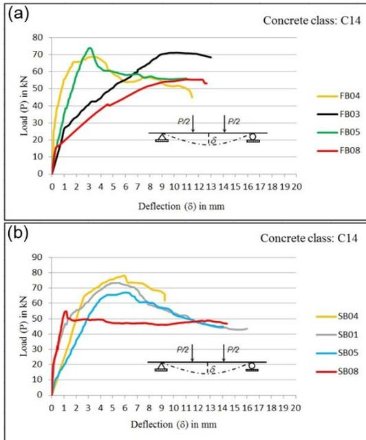
FIGURE 11. Comparison of load-deflection ( $P-\delta$ ) curves for strengthened beams and control beams: (a) FB Series, (b) SB Series.
