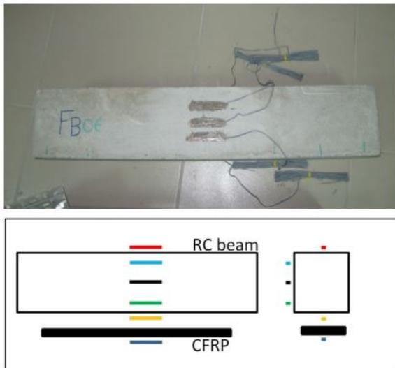
FIGURE 3. The application of strain gauges on beam FB06.
