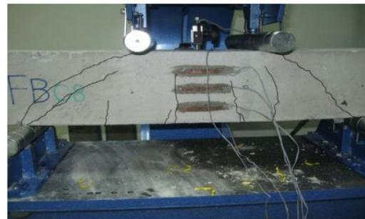
FIGURE 9. Flexural and shear cracks formed in FB08 beam upon loading.
