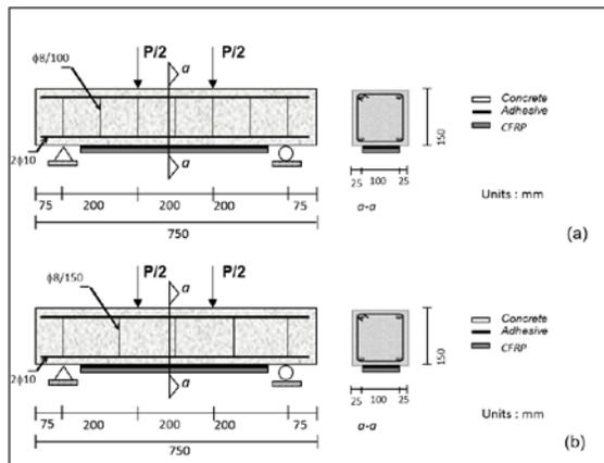
FIGURE 1. The details of the beam series: (a) Flexural beams (FB), (b) Shear beams (SB).
