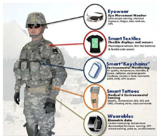
FIGURE 1. Examples of wearable sensor technologies (figure from Ref [3]).
