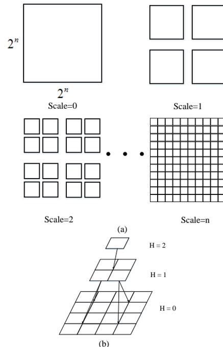
FIGURE 2. (a) Image divided into squares at different scales. Each square can be associated with Haar wavelet coefficients, (b) Hierarchical MRF model.
