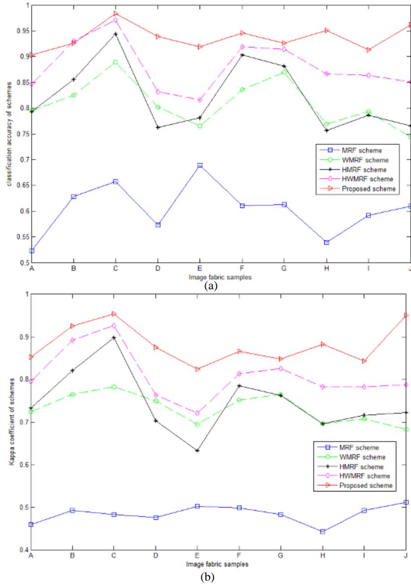
FIGURE 8. Curves of comparison with different methods, (a) classification accuracy of different schemes using 10 images, (b) kappa coefficient of different schemes using 10 images.
