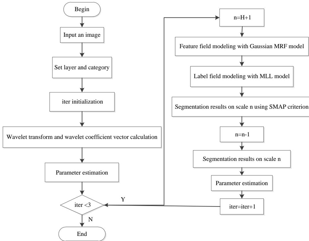
FIGURE 6. The flow chart of proposed algorithm.
