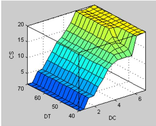
FIGURE 8. Control surfaces of the fuzzy inferring system for color strength at 60°C PT.
