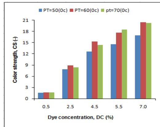
FIGURE 12. Effect of dye concentration and dyeing process temperature on color strength at 60 min DT.
