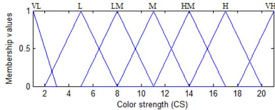
FIGURE 6. Membership functions of output variable CS.
