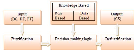
FIGURE 1. Basic configuration of fuzzy logic system [24-26].
