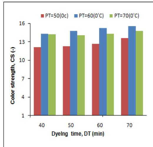
FIGURE 13. Effect of dyeing time and dyeing process temperature on color strength at 4.5% DC.
