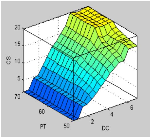
FIGURE 9. Control surfaces of the fuzzy inferring system for color strength at 60 min DT.
