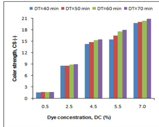
FIGURE 11. Effect of dye concentration and dyeing time on color strength at 60°C PT.
