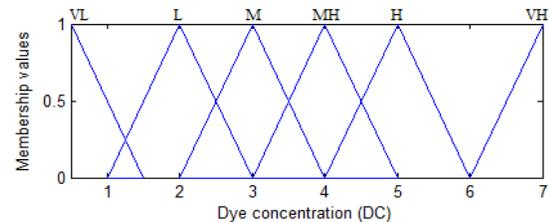
FIGURE 3. Membership functions of input variable DC.
