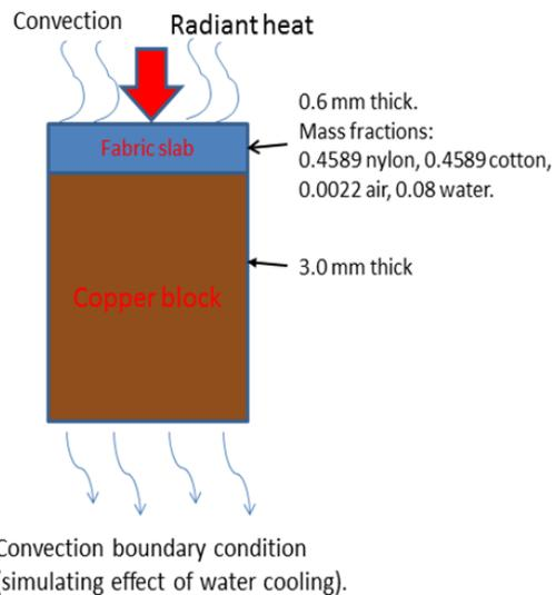
FIGURE 2. Object structure for simulation of test in TBTA.
