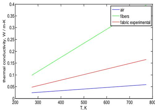
FIGURE 1. Temperature dependence of fiber and air thermal conductivities used in model.
