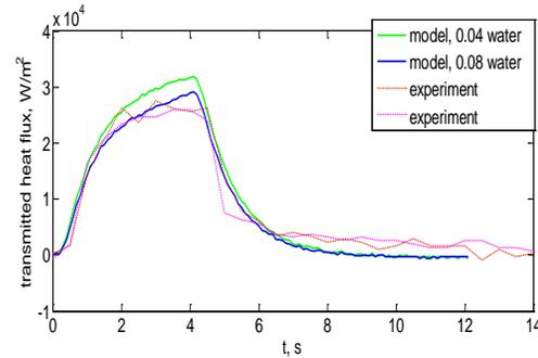
FIGURE 5. Thermal protection test in TBTA,  $77 \text{ kW/m}^2$  incident heat flux, 4 s duration. Solid blue line – model, high moisture. Solid green line – model, moderate moisture. Dotted lines – experiments.
