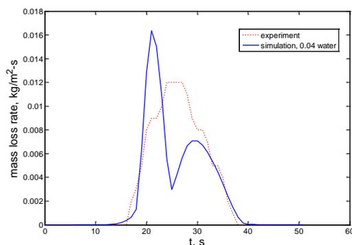
FIGURE 7. Cone calorimeter test, 25 kW/m<sup>2</sup> incident heat flux. Solid blue line – model, moderate moisture. Dashed red line – typical experimental results.
