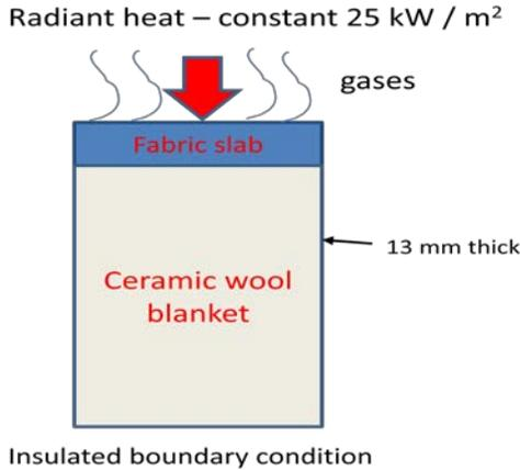
FIGURE 3. Object structure for simulation of flammability test in cone calorimeter.
