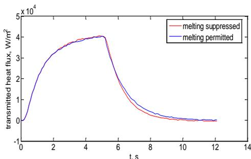
FIGURE 6. Thermal protection test in TBTA, 90 kW/m<sup>2</sup> incident heat flux, 5 s duration. Solid blue line – model, low moisture, nylon melting permitted. Solid red line – model, low moisture, nylon melting suppressed.
