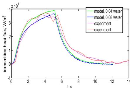
FIGURE 4. Thermal protection test in TBTA,  $90 \text{ kW/m}^2$  incident heat flux, 5 s duration. Solid blue line – model, high moisture. Solid green line – model, moderate moisture. Lines with symbols – experiments.
