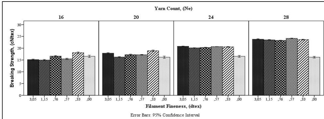
FIGURE 2. Effect of filament fineness on the breaking strength of each yarn count.
