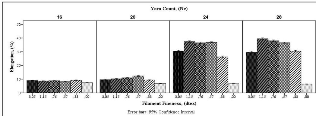
FIGURE 3. Effect of filament fineness on the elongation of each yarn count
