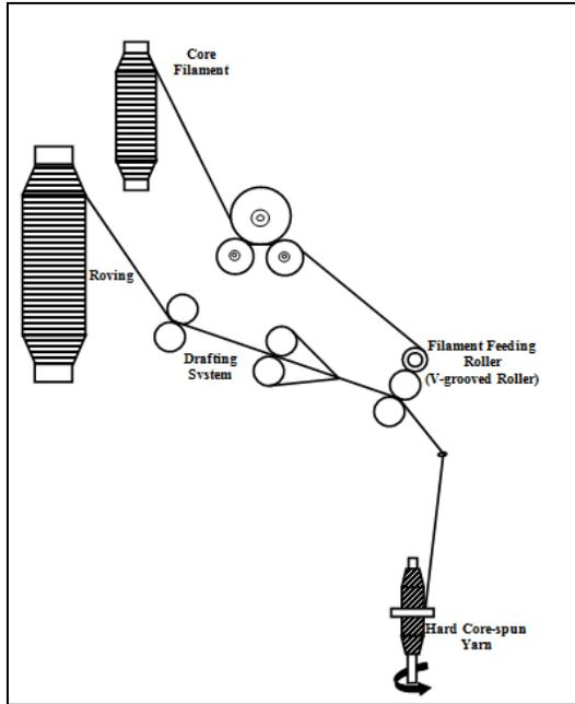
FIGURE 1. Modified ring spinning system [12].
