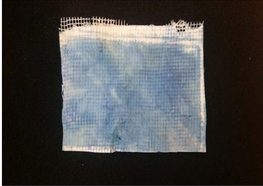
FIGURE 5. Nanofibrous membranes containing TiO<sub>2</sub> nanoparticles after methylene blue removal experiments.
