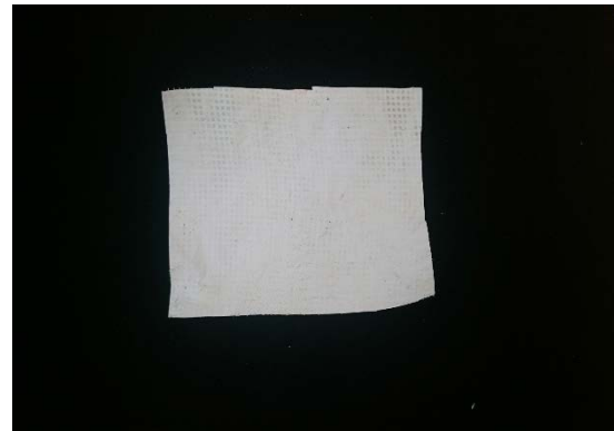
FIGURE 4. Nanofibrous membranes containing TiO_2 nanoparticles before methylene blue removal experiments.
