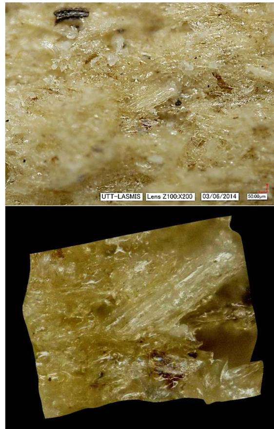
FIGURE 8. Starch matrix structure and 3D representation (50 µm scale X 200).
