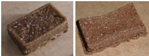
FIGURE 2. Test samples produced using wood pulp.
