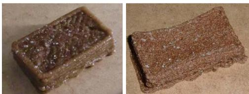
FIGURE 2. Test samples produced using wood pulp.
