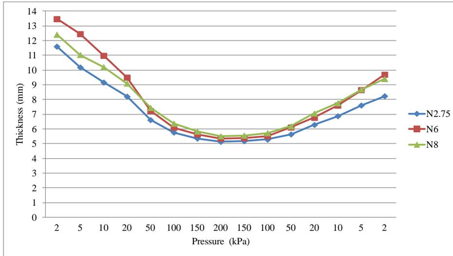
FIGURE 9. Carpet thickness values during loading-unloading treatment.
