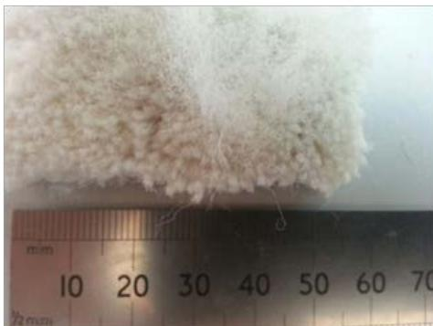
FIGURE 2. Loose fibers and fuzz on the carpet surface.
