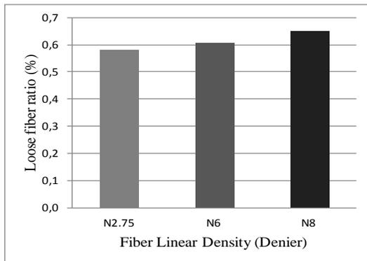
FIGURE 5. Loose fiber ratios versus fiber linear density.
