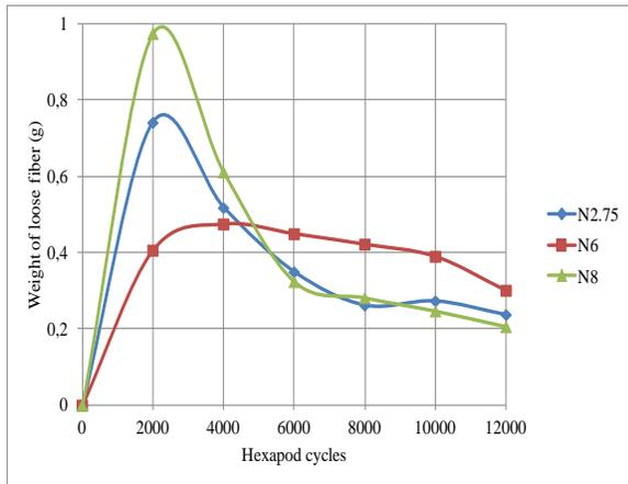
FIGURE 4. Weights of loose fibers versus cycles.
