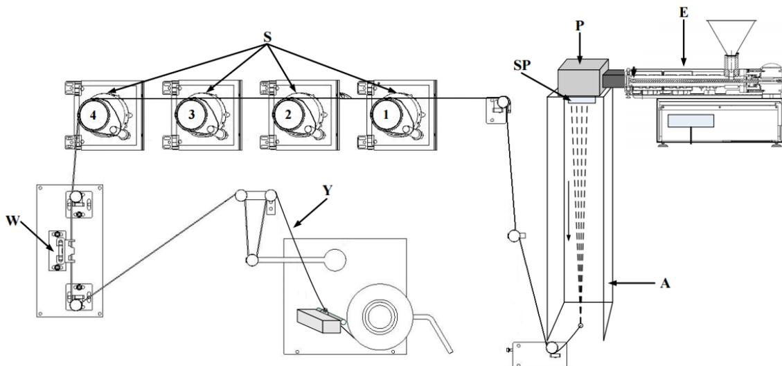
FIGURE 2. Collin CMF 100 melt-spinning system. E: extruder, P: melting pump, SP: spinneret, A: air quench cabinet, S: stretching godets (godet No 1, No 2, No 3, No 4), W: whirling unit, Y: yarn.
