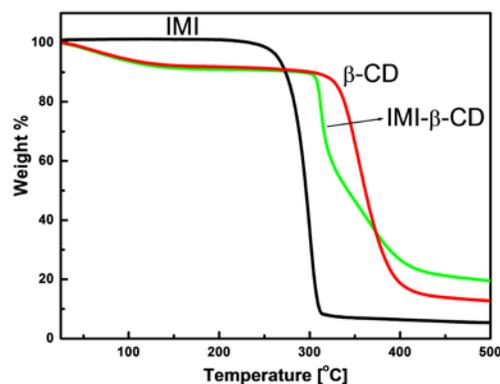
FIGURE 4. TGA graphs of IMI,  $\beta$ -CD and IMI- $\beta$ -CD inclusion complex.
