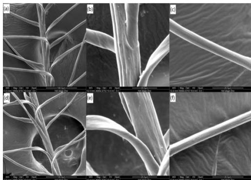
FIGURE 3. SEM micrographs of the surface morphology of unmodified down (a: 1000×, b: 4000×, c: 5000×) and modified down (d: 1000×, e: 4000×, f: 5000×).
