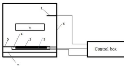
1-temperature sensor, 2-experiment panel, 3-heating panel, 4-shielding panel, 5-insulated panel, 6-experimental box, 7-baseplate, 8-operation window
