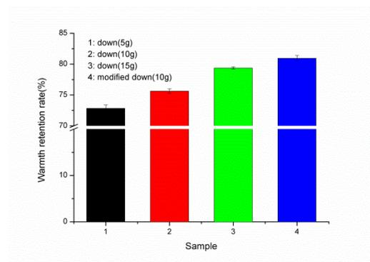
FIGURE 6. The change in the warmth retention rate across different samples.
