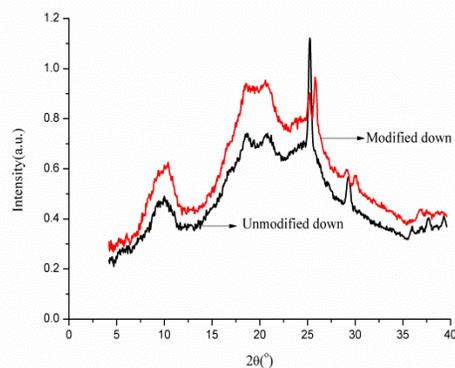
FIGURE 8. X-ray diffractogram of modified and unmodified down.
