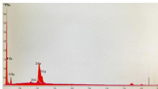
FIGURE 4. EDX spectrum of the modified down.
