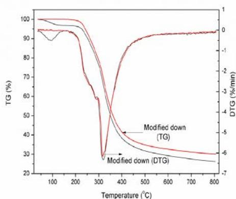
FIGURE 7. TGA/DTG curves of the modified and unmodified down.
