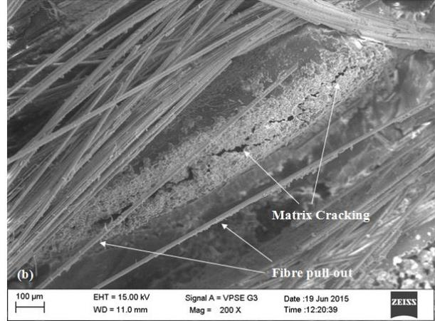
FIGURE 5. SEM image of a) PW composite tensile specimen b) PW composite flexural specimen.
