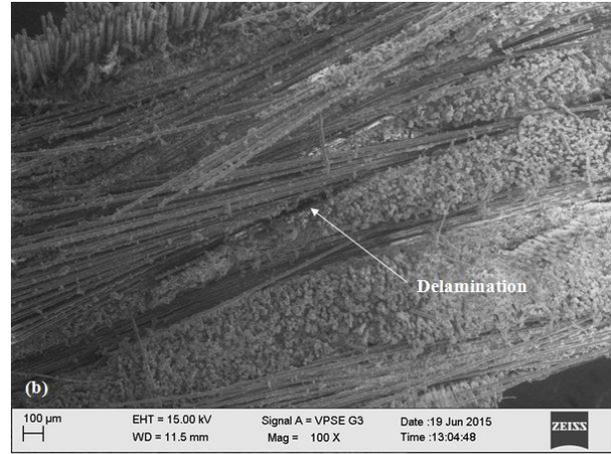
FIGURE 6. SEM image of a) PW composite impact specimen b) PW composite ILSS specimen.
