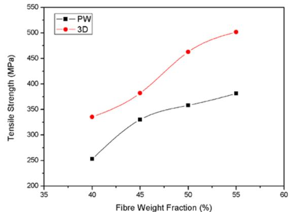
FIGURE 1. Variation in average tensile strength.
