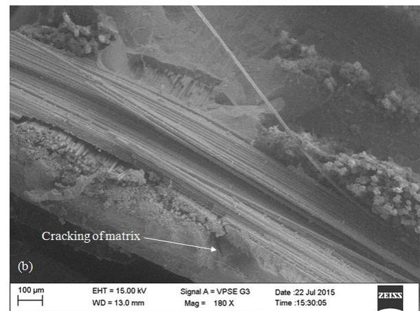
FIGURE 7. SEM image of a) 3D composite tensile specimen b) 3D composite flexural specimen.
