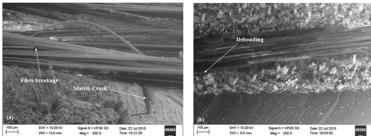
FIGURE 8. SEM image of a) 3D composite impact specimen b) 3D composite ILSS specimen.
