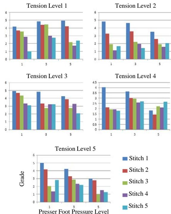
FIGURE 7. Seam pucker grade vs presser foot pressure under fixed tension level
