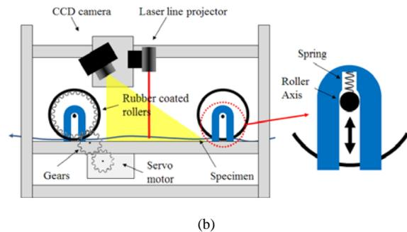
FIGURE 3. Seam pucker measurement system (a) Overview (b) Detailed mechanism.
