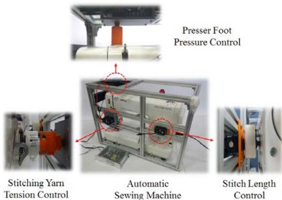
FIGURE 1. Automation of sewing machine.
