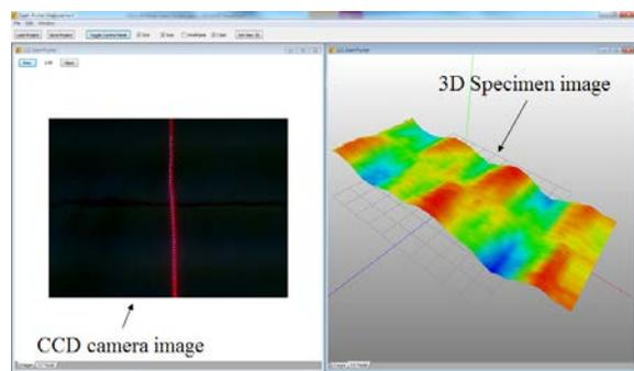
FIGURE 5. Overview of Seam Pucker Measurement software.
