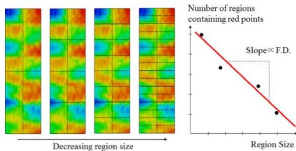
FIGURE 4. Schematic diagram of modified box counting.
