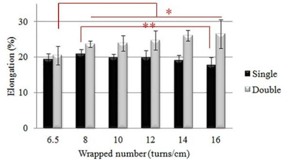
FIGURE 6. Effects of wrapped number and lamination number on tensile elongation of single and double wrapped complex yarns.
