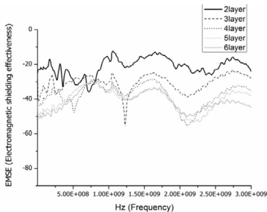
FIGURE 13. Effect of number of layers (2~6 layers) on EMSE of composite fabrics plied with 0°/ 45°/ 90°/ -45°/ 0°/ 45° (weft yarn: sscucu).
