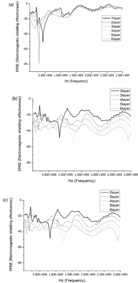
FIGURE 8. Effect of number of layers on EMSE of composite fabrics plied with 0°, 45°, and 90° orientations (wrapped number: 16 turns/cm).
