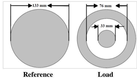
FIGURE 4. Sample holder dimensions for EMI testing [17].
