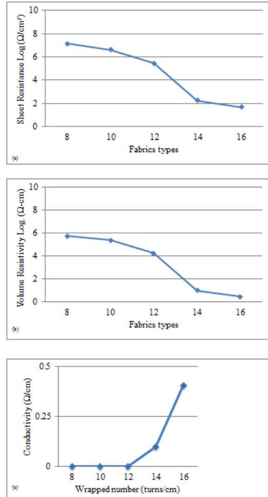
FIGURE 7. Effect of wrapped number on surface resistance (a), volume resistance (b) and conductivity (c) of composite fabrics.
