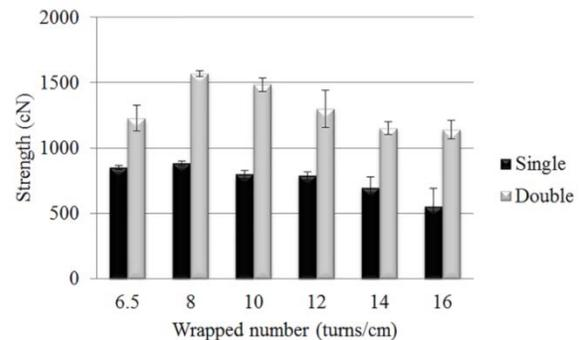
FIGURE 5. Effects of wrapped number and lamination number on tensile strengths of single and double wrapped complex yarns.
