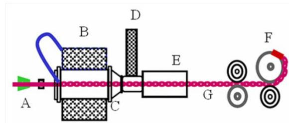
FIGURE 1. The configuration of the rotor twisting machine. A: thread eyes; B: PET yarn; C: a rotor twister; D: tangent belt driven by a motor; E: bearing; F: winding roller; and G: SS/PET complex yarn.
