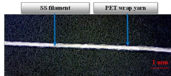
FIGURE 2. Stereomicroscopic observation of SS/PET wrapping yarn. (SS diameter: 0.04 mm, wrap number: 4 turns/ cm, rotor twisting speed: 8000 rpm).
