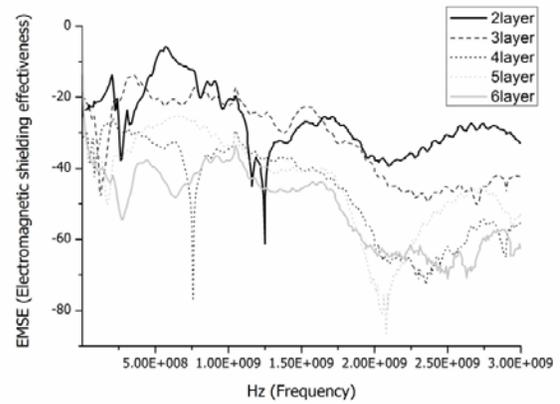
FIGURE 10. Effect of number of layers (2~6 layers) on EMSE of composite fabrics plied with 0°/ 90°/ 0°/ 90°/ 0°/ 90° (weft yarn: cucu005ss).
