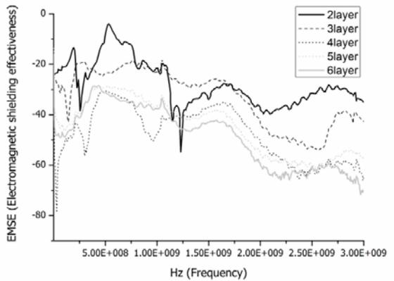
FIGURE 12. Effect of number of layers (2~6 layers) on EMSE of composite fabrics plied with 0°/ 90°/ 0°/ 90°/ 0°/ 90°(weft yarn: cucu008ss).
