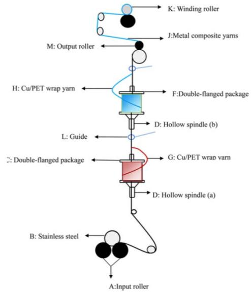
FIGURE 3. Spinning diagram of single and double wrapped complex yarn.
