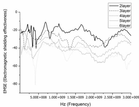
FIGURE 9. Effect of number of layers on EMSE of composite fabrics plied with 0°/45°/90°/-45°/0°/45°(weft yarn: cucu005ss).
