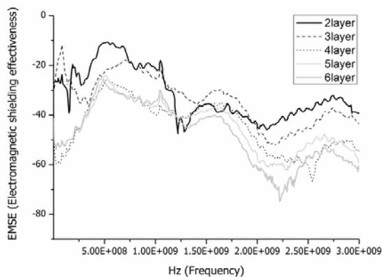
FIGURE 14. Effect of number of layers (2~6 layers) on EMSE of composite fabrics plied with 0°/ 90°/ 0°/ 90°/ 0°/ 90° (weft yarn: sscucu).
