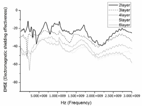
FIGURE 11. Effect of number of layers (2~6 layers) on EMSE of composite fabrics plied with 0°/ 45°/ 90°/ -45°/ 0°/ 45° (weft yarn: cucu008ss).
