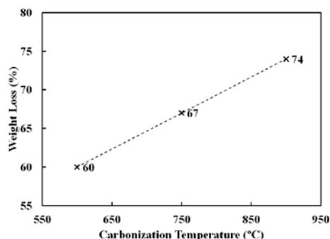
FIGURE 4. The weight loss of SFSL-based carbonized fibers (L1) as a function of carbonization temperature
