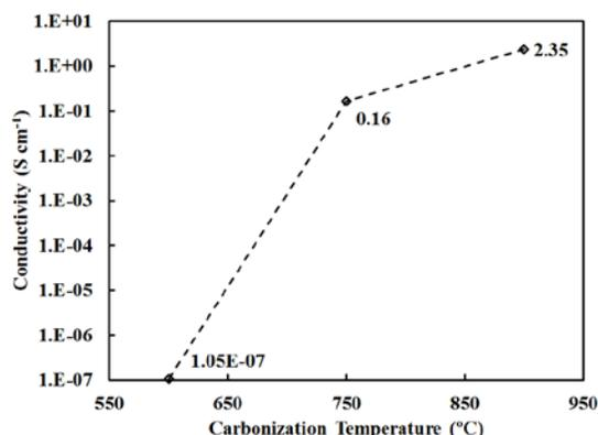
FIGURE 8. Electrical conductivity of SFSL-based carbonized fibers (L1) as a function of carbonization temperature.
