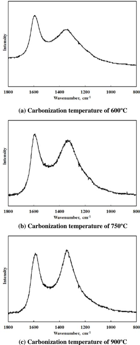
FIGURE 5. Raman spectra of SFSL-based carbonized fibers (L1).
