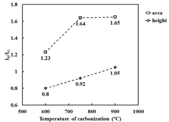
FIGURE 6. The ratio of D-peak to G-peak ( $I_D/I_G$ ) of SFSL-based carbon fibers (L1). ( $I_D/I_G$ ) calculated from Raman spectra based on height and area of peaks.
