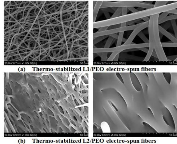
FIGURE 1. SEM images of thermo-stabilized (a) L1/PEO and (b) L2/PEO electro-spun fibers. The heating rate was 1°C/min from room temperature to 250°C and holding isothermally 1 h in air atmosphere. (left and right image scales are 50 and 10 micrometers, respectively).
