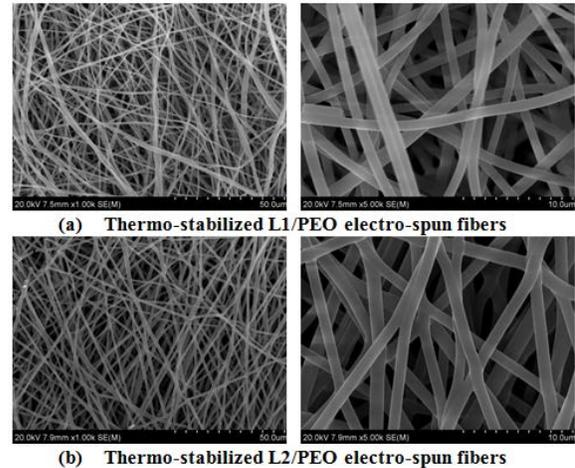
FIGURE 2. SEM images of thermo-stabilized (a) L1/PEO and (b) L2/PEO electro-spun fibers. The heating rate is 0.5°C/min from room temperature to 250°C and holding isothermally 1 h in air atmosphere. (left and right image scales are 50 and 10 micrometers, respectively).
