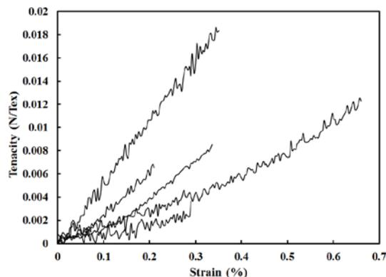
FIGURE 9. Typical stress-strain curves of SFSL-based carbonized fibers (L1) at a carbonization temperature of 900°C.
