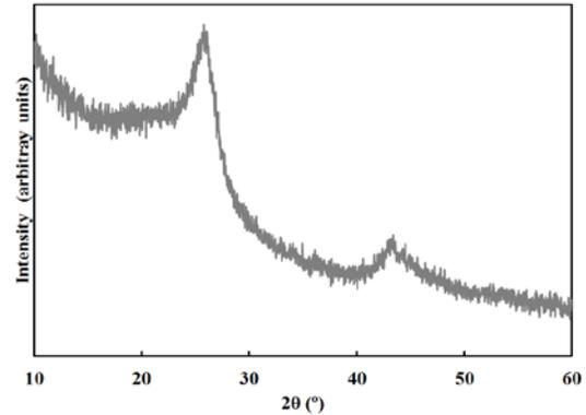
FIGURE 7. X-ray diffraction patterns of SFSL-based carbonized fibers (L1).
