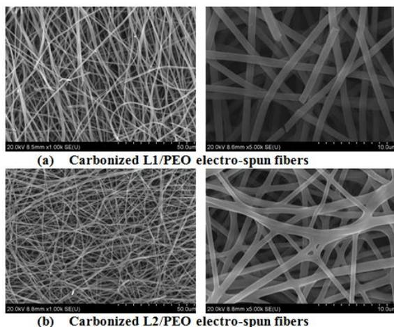
FIGURE 3. SEM images of carbonized (a) L1/PEO and (b) L2/PEO electro-spun fibers. The heating rate is 0.5°C/min from room temperature to 250°C and holding isothermally 1 h in air atmosphere, then the heating rate is 5°C/min from 250°C to 900°C and holding isothermally 1 h in Argon atmosphere. (left and right image scales are 50 and 10 micrometers, respectively).
