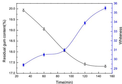
FIGURE 4. Effect of system time on the residual gum content and the whiteness of flax rove in supercritical carbon dioxide fluid. (-Δ-) Residual gum content, (-■-) Whiteness.
