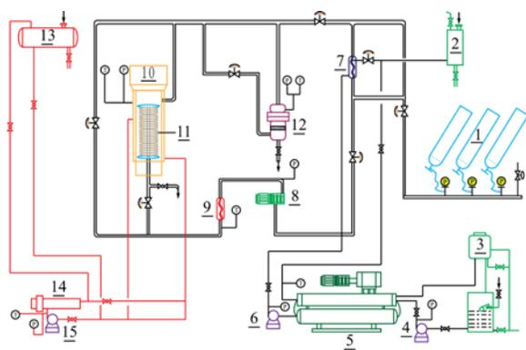
FIGURE 1. Schematic diagram of supercritical carbon dioxide fluid apparatus for scouring and bleaching: (1) carbon dioxide cylinder, (2) ethylene glycol elevated tank, (3) cooling tower, (4) water pump, (5) compressor, (6) ethylene glycol pump, (7) refrigerator, (8) high-pressure pump, (9) heat exchanger, (10) scouring and bleaching vessel, (11) flax rove, (12) separator vessel, (13) conduction oil tank, (14) conduction oil system, (15) oil pump.
