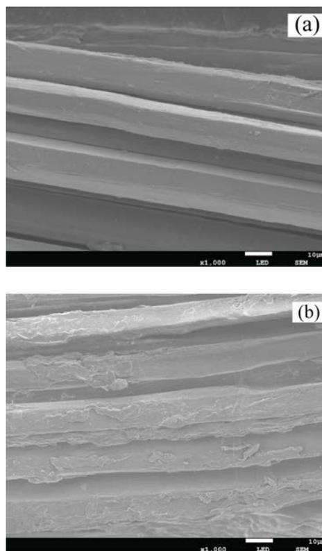
FIGURE 6. SEM images of the flax rove: fiber surface of the original sample (a) treated at a temperature of 120°C (b) in supercritical carbon dioxide fluid.
