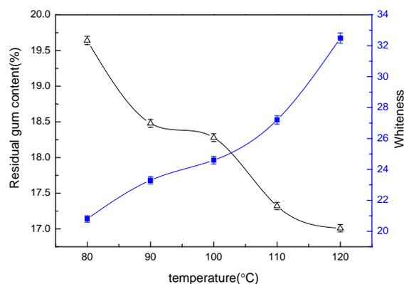
FIGURE 2. Effect of system temperature on the residual gum content and the whiteness of flax rove in supercritical carbon dioxide fluid. (-Δ-) Residual gum content, (-■-) Whiteness.
