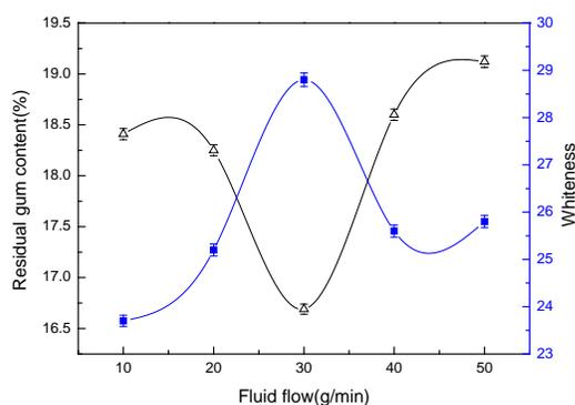
FIGURE 5. Effect of fluid flow on the residual gum content and the whiteness of flax rove in supercritical carbon dioxide fluid. (-Δ-) Residual gum content, (-■-) Whiteness.
