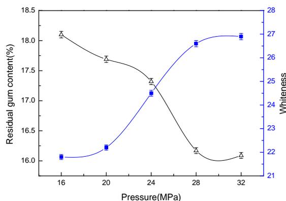
FIGURE 3. Effect of system pressure on the residual gum content and the whiteness of flax rove in supercritical carbon dioxide fluid. (-Δ-) Residual gum content, (-■-) Whiteness.
