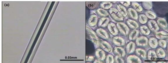
FIGURE 1. The optical microscope images of the ECDP-H (a) longitudinal morphology and (b) cross-section.
