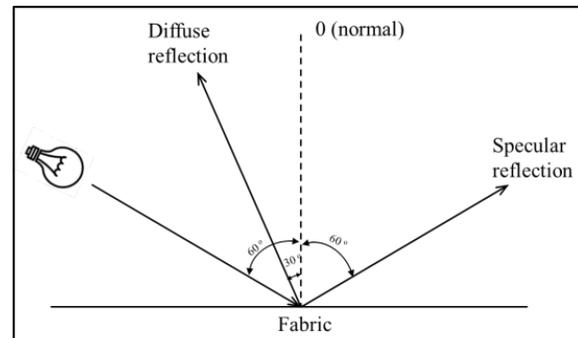
FIGURE 2. Schematic diagram of fabric glossiness test.
