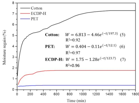
FIGURE 3. Dynamic moisture absorption curves of fabrics.
