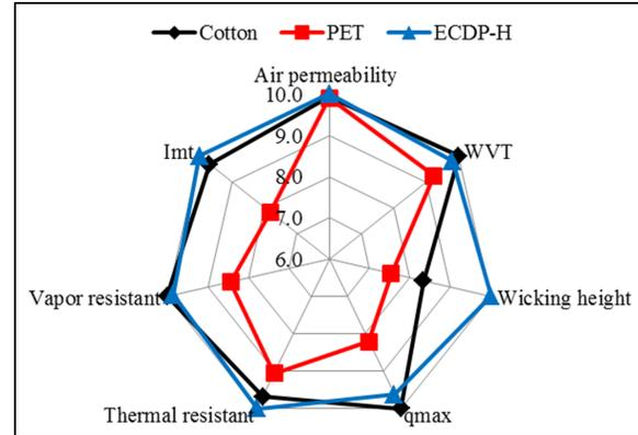
FIGURE 4. Radar plot for comparisons of fabrics comfort properties.
