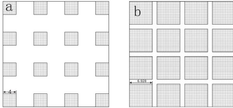
FIGURE 1. Illustration of fabrics coated with the same numbers of small silicone squares but different coating area (a) 25% coating area, (b) 75% coating area.(Shadow: silicone coating).
