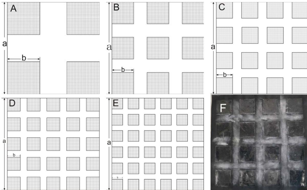
FIGURE 2. Illustration of fabrics coated with the same coating area but different numbers of small silicone squares (A)2x2,(B)3x3,(C)4x4,(D)5x5,(E)6x6,(F)The photo of fabric coated with 4x4 small silicone square.
