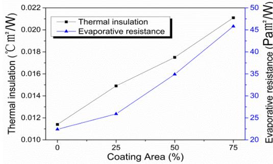
FIGURE 3.  $R_{ct}$  and  $R_{et}$  of samples with different coating areas.
