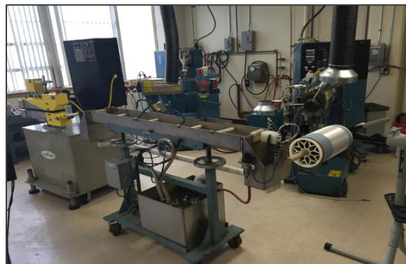
FIGURE 6. Apparatus for continuous GP extraction process: (left) fiber puller system. (center) water bath, and (right) fiber pay-off system.
