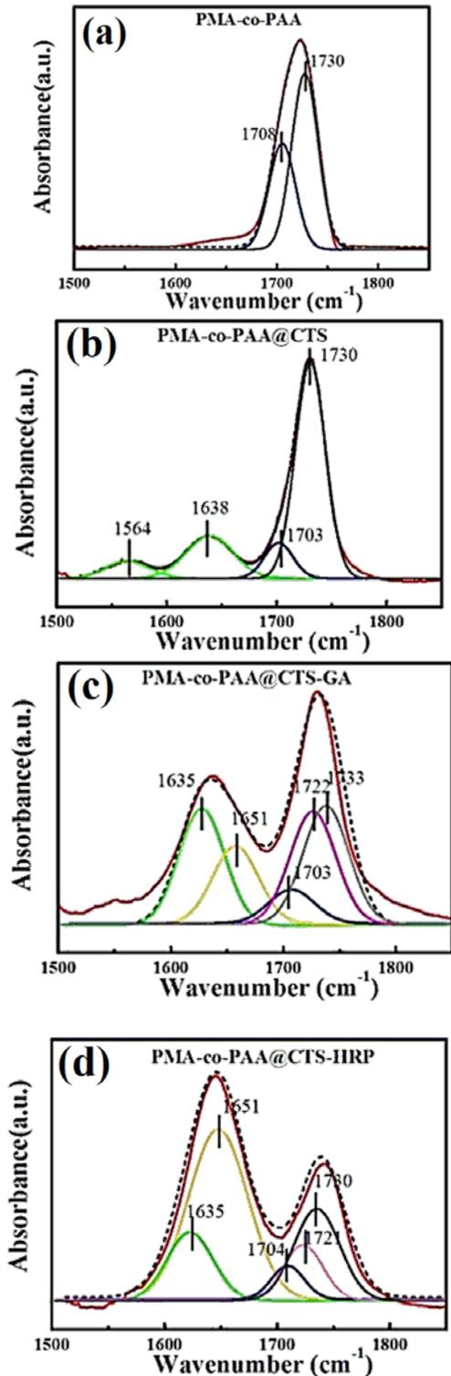
FIGURE 4. FTIR spectra of the pristine PMA-co-PAA (a), PMA-co-PAA@CTS (b), PMA-co-PAA@CTS-GA(c), PMA-co-PAA @ CTS-HRP (d), respectively.
