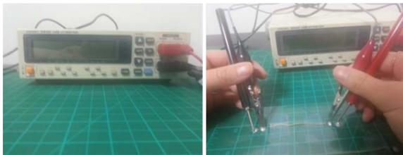
FIGURE 4. Conductivity measurement of Conductive Yarns Using a Low Ohm Meter.
