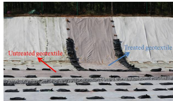
FIGURE 5. Untreated and tread geotextiles in weathering test.
