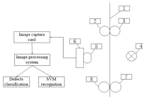
FIGURE 1. Schematic of the raw-silk defect detection and recognition system.
