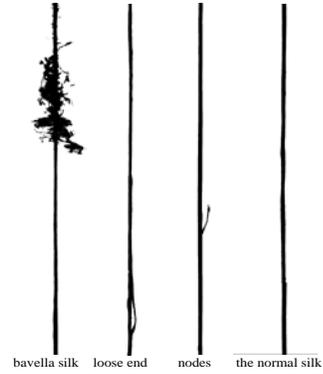
FIGURE 7. Image taken after threshold segmentation.
