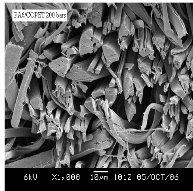
Figure 10. SEM photo of PA6/COPET fiber web cross-section after hydroentanglement
