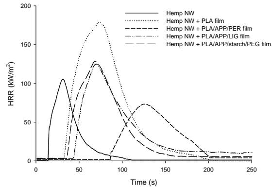
FIGURE 3. HRR as a function of time for samples with hemp nonwoven (external heat flux= 35 kW/m<sup>2</sup>)
