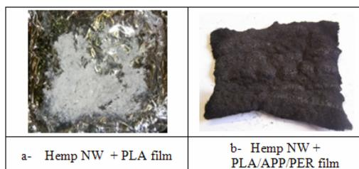
FIGURE 4. Residues of hemp NW + PLA film and hemp NW + PLA FR film after a test carried out with the cone calorimeter (35 kW/m<sup>2</sup>)
