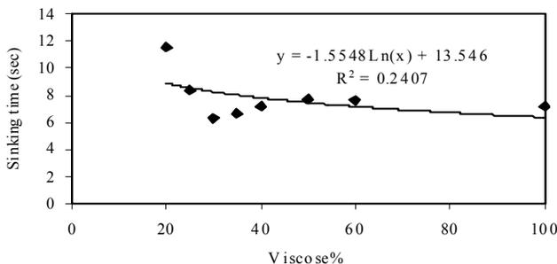
FIGURE 3. Effect of viscose proportion on sinking time
