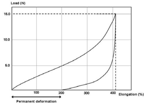
FIGURE 4. Fabric cyclic loading diagram.
