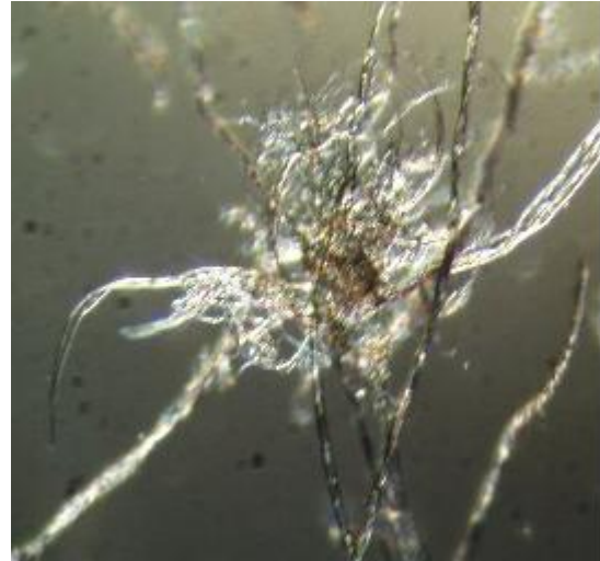
FIGURE 2. Frayed fiber in suspension
