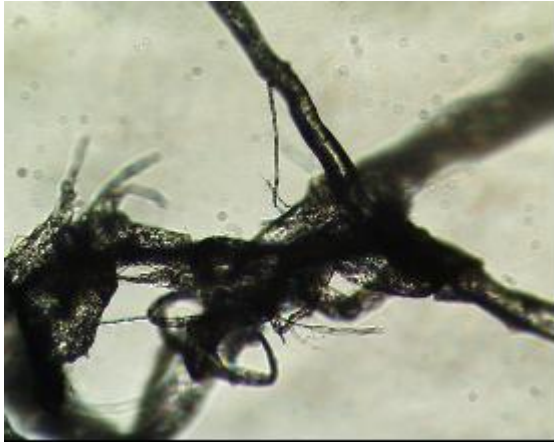
FIGURE 11. Frayed point comprised of tow fibers
