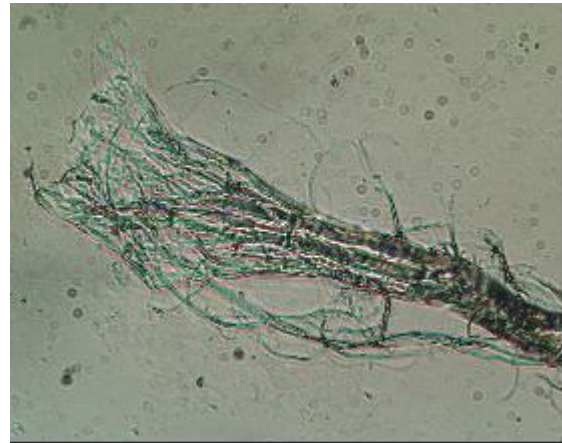
FIGURE 10. Frayed point comprised of single fiber is a frayed fiber cut site indeed.
