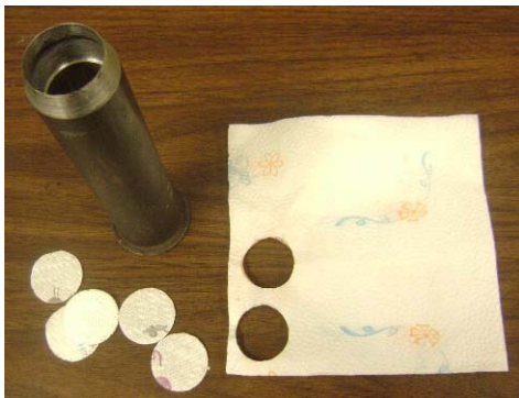
b) The tool that was used to cut the wipes
