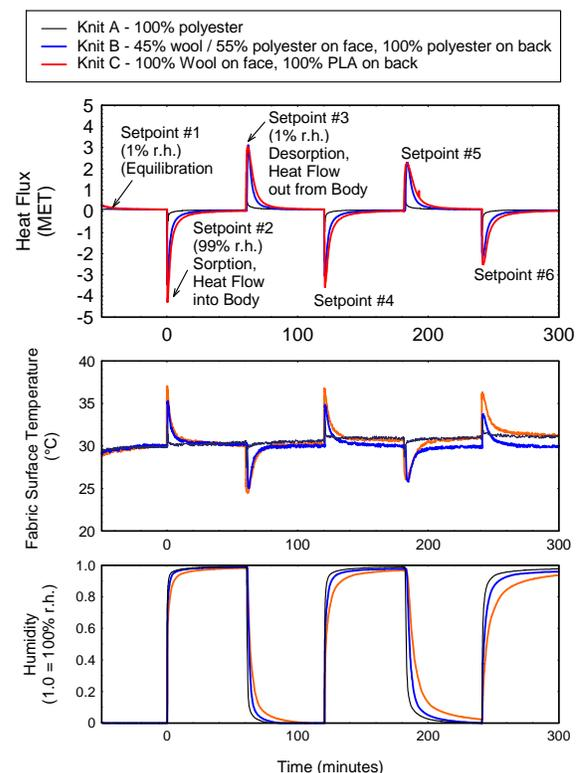
FIGURE 5. Heat flux, temperature, and humidity measurements from flow cell under step changes in relative humidity.
