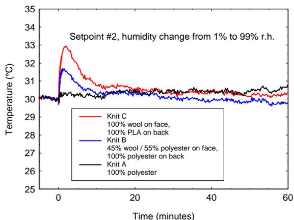
FIGURE 6. Relative temperature change from ambient temperature underneath the fabrics during step changes in humidity.
