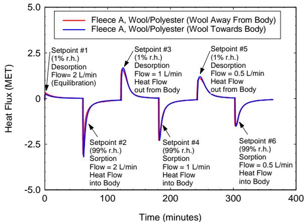
FIGURE 8. Effect of the orientation of the wool side of the wool/polyester thick fleece fabric (Fleece A) on heat flux due to water vapor sorption.
