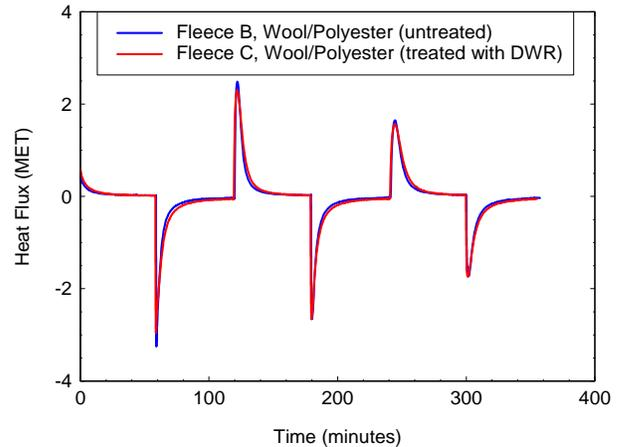
FIGURE 9. The heat flux sensor data for the comparison of a fleece fabric with a DWR treatment (Fleece C) with the same fabric without a DWR treatment (Fleece B).
