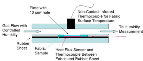
FIGURE 4. Test cell setup to observe temperature and heat flow for fabrics subjected to a step change in relative humidity.
