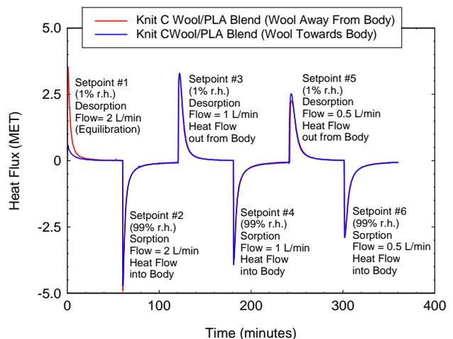
FIGURE 7. Effect of the orientation of the wool side of the 100% Wool / 100% PLA thin knit fabric (Knit C) on the heat flux due to water vapor sorption.
