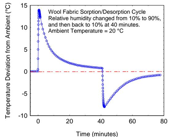
FIGURE 3. Temperature change in wool fabric due to water vapor sorption.
