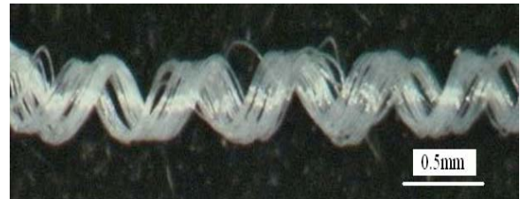
FIGURE 8. Configuration of new PTT/PET after wet-heat treatment
