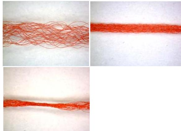
FIGURE 9. The Geometrical structure of set, stretch and intermingled yarn.
