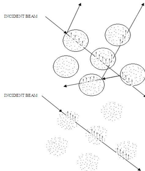
FIGURE 3. Scattering of light by fibers.
