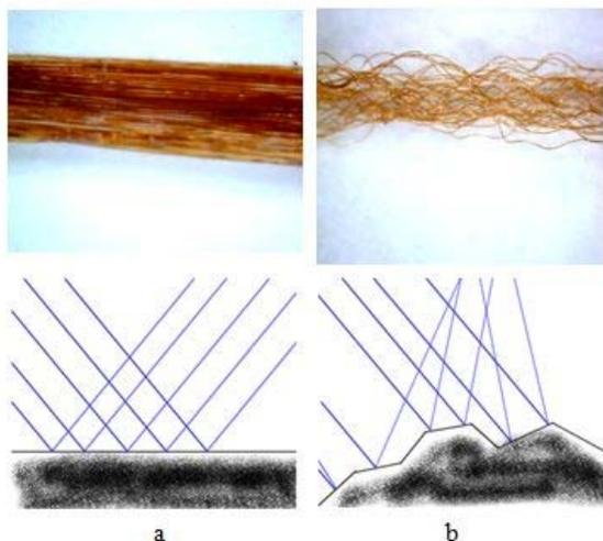
FIGURE 4. Geometrical structure of a) POY and b) textured yarn.
