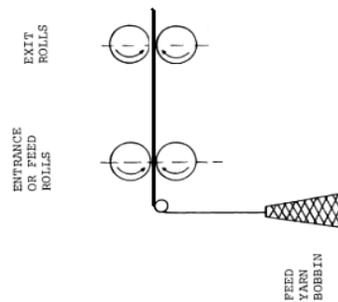
FIGURE 2. Schematic of drawing unit.
