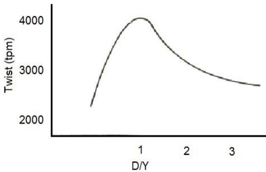
FIGURE 8. Variations of twist with D/Y ratio.
