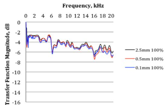
FIGURE 5. The Effect of The Diameter of Glass Beads on Sound Insulation.
