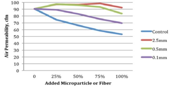
FIGURE 2. Air permeability results of glass beads or fiber added nonwovens. C: Control Fabric, 2.5mm: Particle of 2.5mm diameter added nonwoven fabric, 0.5mm: Particle of 0.5mm diameter added nonwoven fabric, 0.1mm: Particle of 100-micron diameter added nonwoven fabric.
