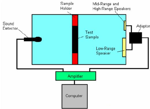
FIGURE 1. Illustration of the Clemson–Boston Differential Sound Insulation Tester [5].
