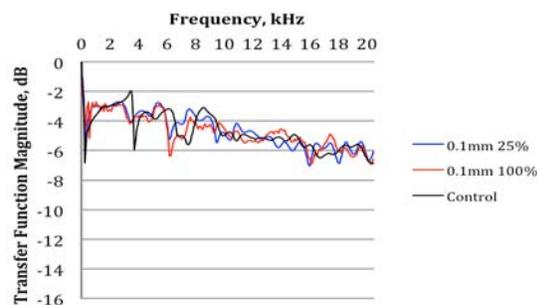
FIGURE 4. The Effect of the Amount of Glass Beads on Sound Insulation
