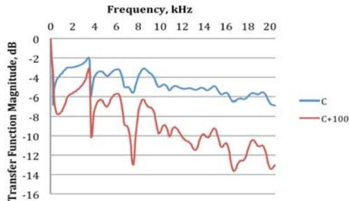
FIGURE 3. The Effect of Fiber Weight on Sound Insulation. C: Control Fabric, C+100: Double weight of control fabric.
