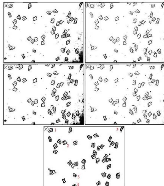
FIGURE 7. Segmentation for the image in *Figure 1* by *Otsu* (a), 1-D Entropy (b), 2-D Entropy (c), and Minimum Error (d) and dual-thresholding (e) algorithms.
