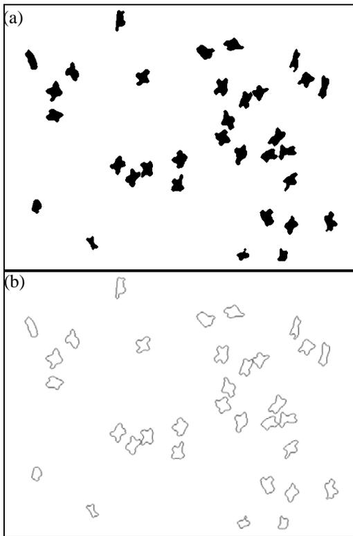
FIGURE 8. Detected fibers (a) and boundaries (b) after removing fiber borders.
