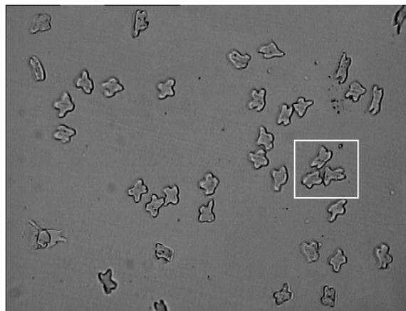
FIGURE 1. Fiber cross-section image from Nikon 50i light microscope system.
