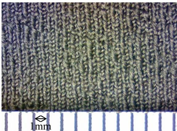
FIGURE 3. BC/S complex fabrics laid-in knitted fabric from BC/S complex yarns.
