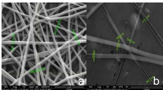
FIGURE 6. SEM image of (10 cm, 11 kV) electrospun nanofibers a) Horizontal system, Syringe with regular needle, 15 kV, Flow rate of 1.6 ml/h, 80 - 150 nm fiber diameter, 50000X b) Vertical system, Syringe with straightened needle tip, 11 kV, 4 ml/h, 70 - 220 nm fiber diameter, 60000X.
