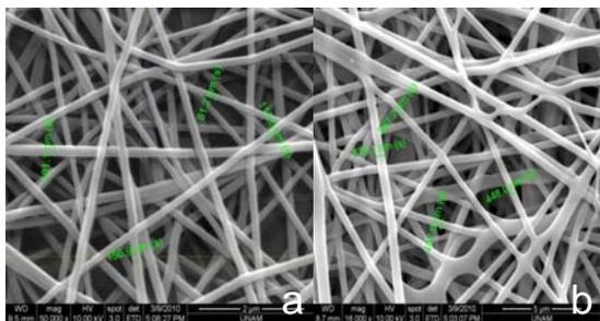
FIGURE 5. SEM images of (horizontal setup, 10 cm, flow rate of 1.6 ml/h) electrospun nanofibers a) 15 kV, 10 %wt PVA, 80-150 nm fiber diameter, 50000X b) 17 kV, 15 %wt PVA, 70-220 nm fiber diameter, 16000X.
