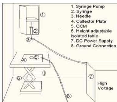
FIGURE 2. Vertical electrospinning setup.
