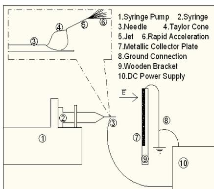
FIGURE 1. Diagram of horizontal electrospinning setup and the droplet shape in detail.
