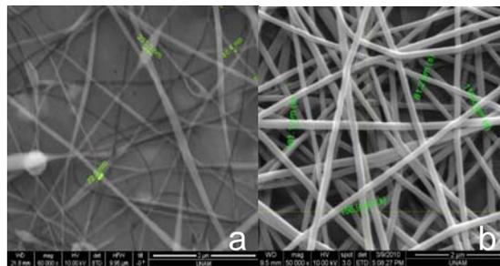
FIGURE 4. SEM images of (10 cm, 15 kV, horizontal setup) electrospun nanofibers a) flow rate of 6 ml/h , 4070 nm fiber diameter, 250 nm bead diameter b) flow rate of 1.6 ml/h, 80-150 nm fiber diameter, non-beaded structure
