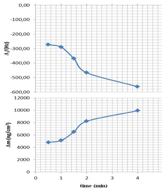
FIGURE 9. Vertical electrospinning system (15 kV- 0.5 ml/h) graphics of time versus a) frequency change ( $\Delta f$ -t) b) mass change ( $\Delta m$ -t).
