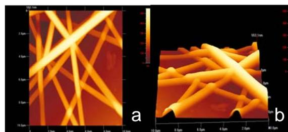
FIGURE 7. AFM images of PVA nanofiber modified gold surface, 10 cm distance between tip and collector, needle diameter of 0.80 mm, 10 %wt PVA, 80°C, 13kV, 0.5 ml/h, a) 2D view b) 3D view.
