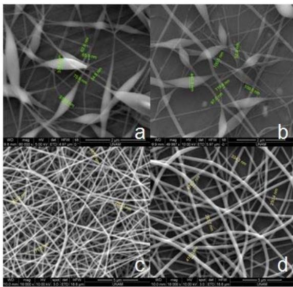
FIGURE 3. SEM images of (10 cm, 12 kV, horizontal setup) electrospun nanofibers a) flow rate of 10 ml/h, 30-60 nm fiber diameter, 300 nm bead diameter, b) flow rate of 6ml/h, 50-100 nm fiber diameter, 440 nm bead diameter, c) flow rate of 1.6 ml/h, 170-220 nm fiber diameter, non-beaded structure d) flow rate of 1.1 ml/h, 230-476 nm fiber diameter, non-beaded structure.
