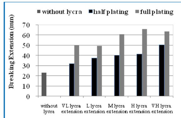
FIGURE 10. Effect of the Lycra extension % on the breaking extension for half, full plating and without Lycra fabrics.
