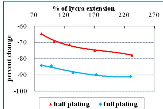
FIGURE 7. Effect of the lycra extension % on the air permeability for dyed fabrics in half and full plating.
