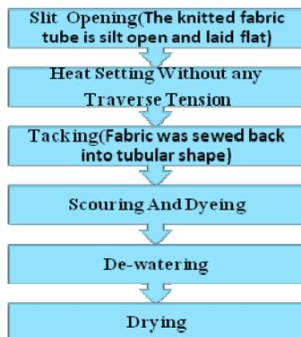
FIGURE 3. Fabric finishing plan.
