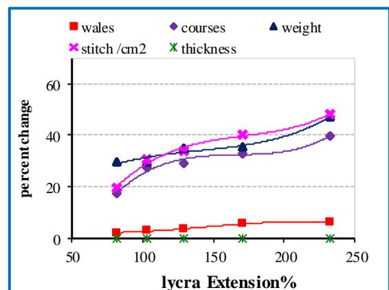
FIGURE 4. Effect of the lycra extension % on the geometrical Properties for half plating dyed fabrics.
