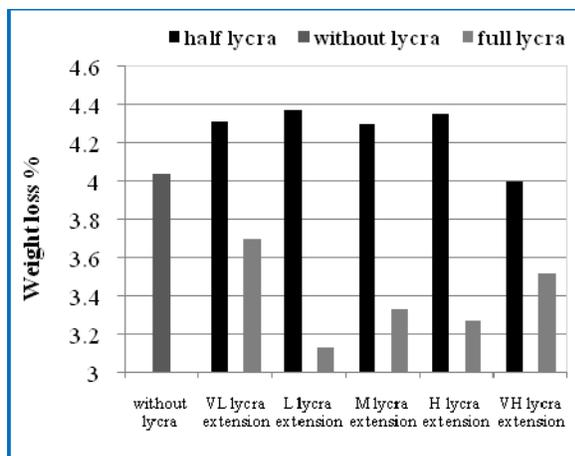
FIGURE 12. Effect of the lycra extension % on the fabric abrasion resistance for dyed samples in half, full plating and without Lycra.
