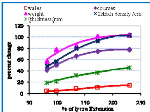
FIGURE 6. Effect of the Lycra extension % on the geometrical Properties for full plating dyed fabrics.
