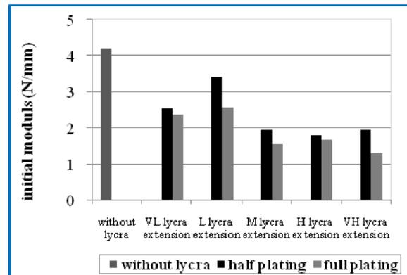
FIGURE 11. Effect of the Lycra extension % on the initial elasticity modulus for half and full plating and without Lycra fabrics.
