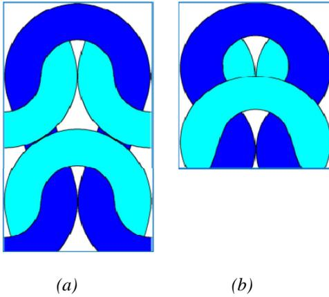
FIGURE 5. Loop structure diagram of the 100% cotton single jersey fabric: (a) theoretical jamming, (b) stitch overlapping.
