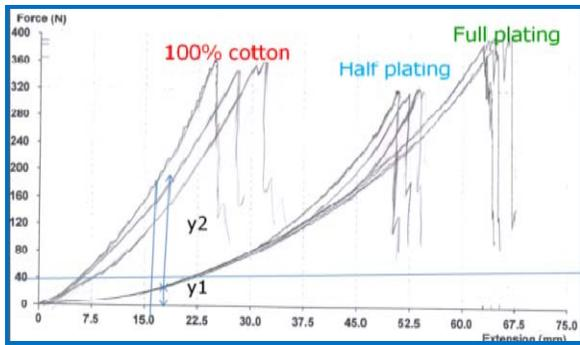
FIGURE 8. Relation between the force and extension result from the bursting strength tester for 100% cotton, half and full plating fabrics.
