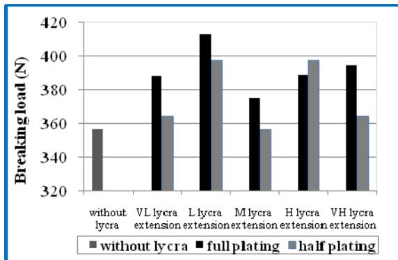
FIGURE 9. Effect of the Lycra extension % on the breaking load for half and full plating and without lycra fabrics.
